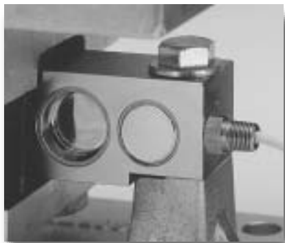
Laser-fused stainless steel cavity covers provide a true hermetic seal.
