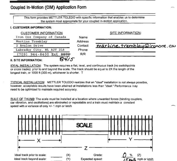
Supply other site information, such as track layout and elevation plans, that may be helpful in determining the proper location of the CIM scale
