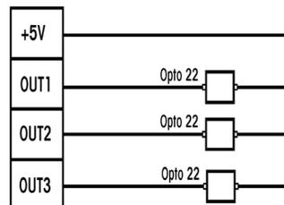
The discrete outputs may be used in conjunction with either the setpoint mode or over/under mode.
