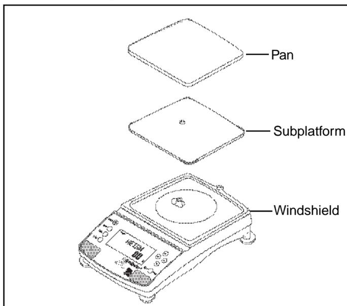
All balances are supplied with a subplatform and pan. The subplatform fits through the hole on top of the balance and rests on a cone assembly which is part of the measuring load cell.
