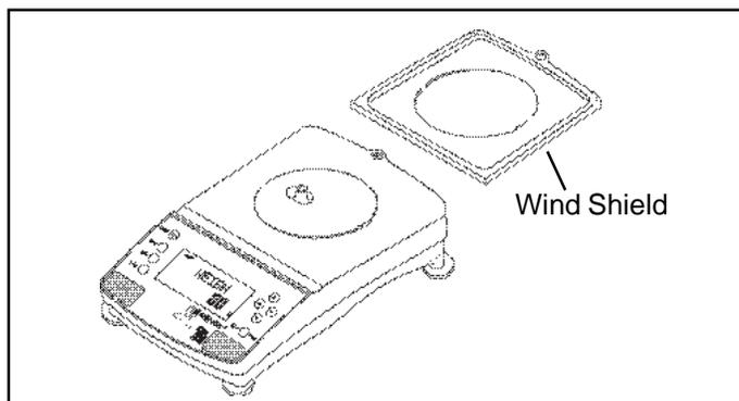
On 810g to 8100g balances, a wind shield is provided to reduce the possibility of air currents from disturbing the pan. When the wind shield is in place, air currents are deflected up over the pan. Place the wind shield on top of the balance making sure the small alignment tab is located properly on the balance.
