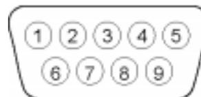
RS-232 Connector Pin Layout.
