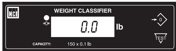
If the display indicates a slightly "off" zero condition (either a number in the display or dashes at the bottom of the display), press the **ZERO** key. When the display shows 0.0, it is ready to weigh.
