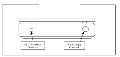
Select an unused Serial DE-9 Communication Port located on the back of your PC (COM 1, 2, 3 or 4) and attach the communication cable provided to your PC. Attach the other end of the communication cable to the 7010SB scale in the SMALL plug jack located in the rear of the unit. See below:
