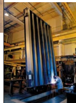
Module positioner allows all welds to be placed in the flat position
