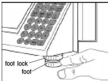
Adjust the four feet until the bubble is in the center of the bubble level. Then adjust the foot locks until the feet are fixed.
