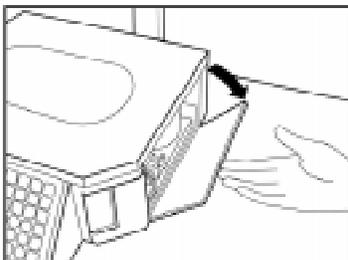
Remove the adhesive tape on the plastic door on the right side of the scale, and open the door.
