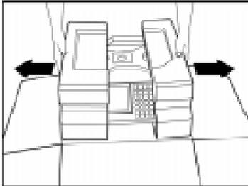
Open up the package box. Take out the platter first, then take out the scale. Take off the foam inserts and plastic bag. Put the scale on the working counter.
