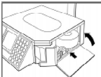
Slide the printer into the scale. Close the plastic door.
