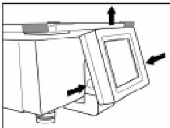
Press two buttons, which are at the two sides of the back display base. Then release the back display from base.
