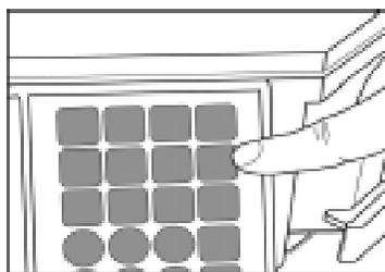
Press the FEED LABEL key to bring the label into the start position.
