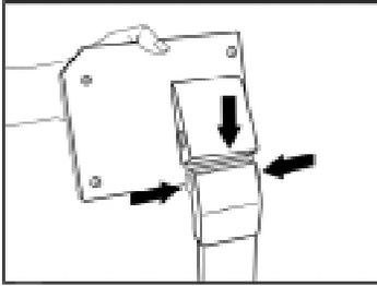
Press the buttons, which are on the sides of the tower. Then insert the back display.
