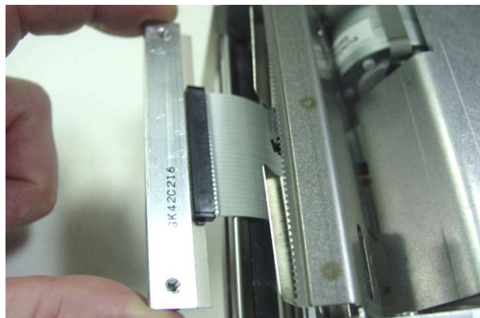
Figure 4-37: Slide Printhead out the Front and Disconnect the Harness
