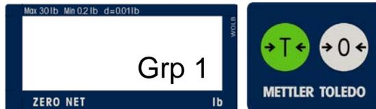
You can press the Tare key to move to Grp 2, 3, 4 or 5. To go into a particular Group, press the Zero Key. Below is what you will see when going into the first Step of Group 1.
