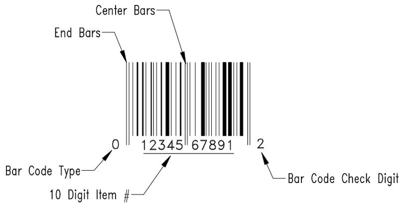
**Figure 7-15 Standard Type 0 Bar Code**
