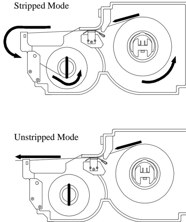
**Figure 4-3 Installing Labels**
