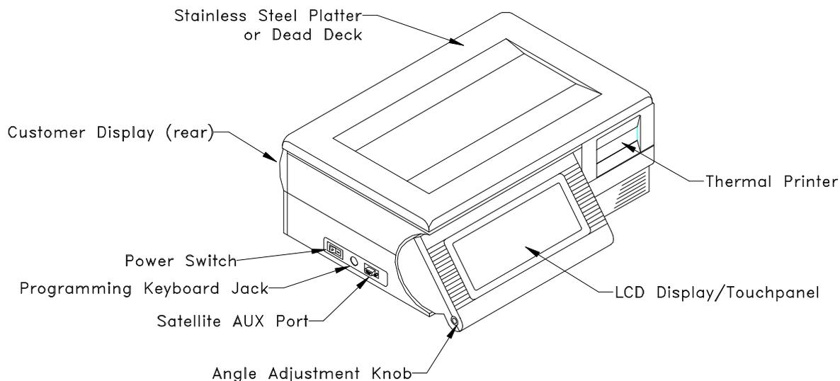
**Figure 2-5 Operator Controls**
