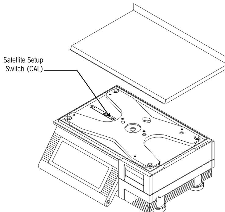
**Figure 7-12 Satellite Setup Switch (CAL)**
