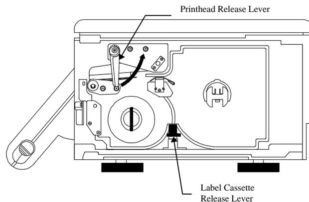
**Figure 4-2 Removing Label Cassette**
