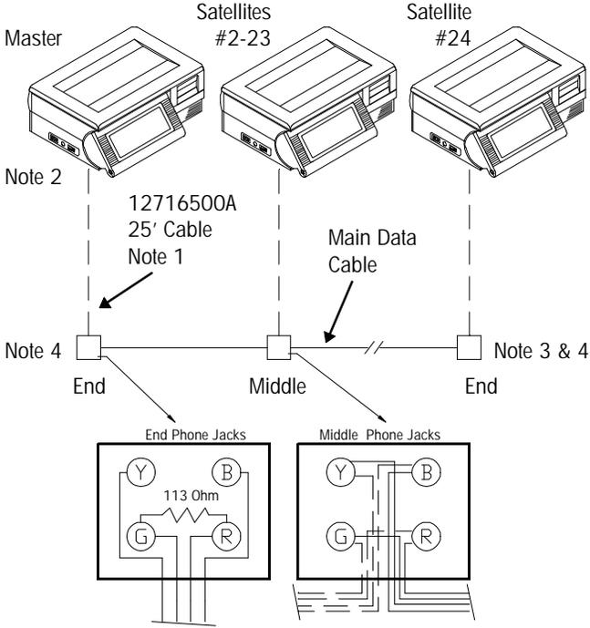
Figure 2-3 - TNET Wiring
