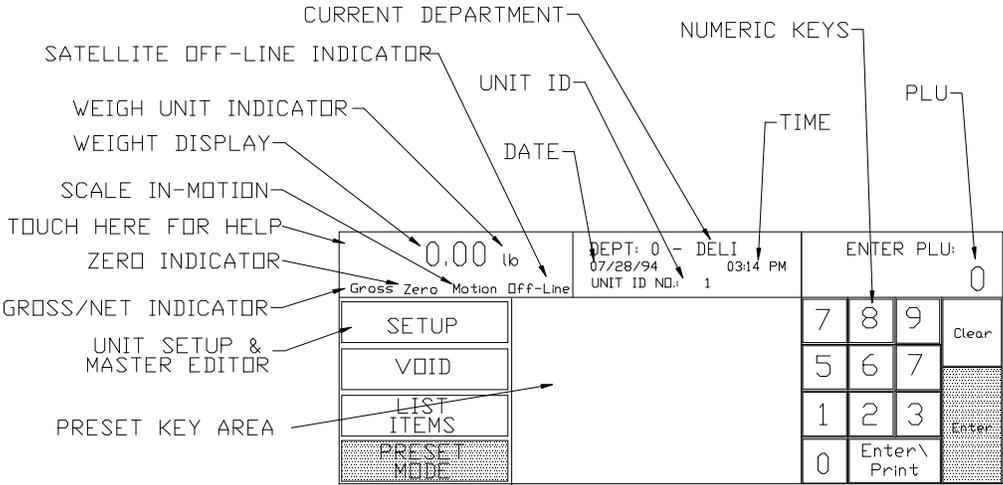
Figure 2-6 Operator Numeric Entry Screen
