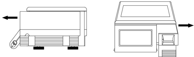
**Figure 4-1 Removing Printer Access Cover.**
