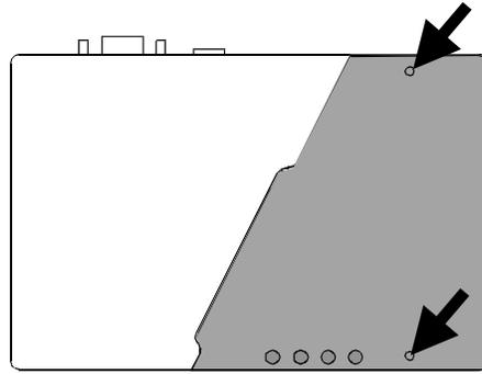
Next, slide the PCMCIA card out from the adapter. Disconnect the antenna leads from the card. Reconnect the antenna leads to the new radio card, then slide the new radio card in the adapter. Push the card in until you can feel the card plug into the receptacle. Route the antenna leads out the top of the adapter and on top of the strain relief block so they are clamped in place when the cover is installed (see below).
