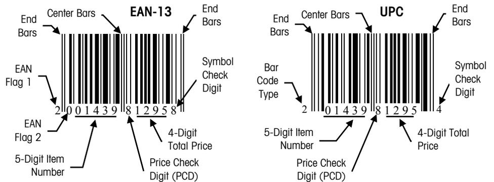
**Figure 1-13: Bar Code Symbols/Price Check Digit (PCD) Enabled**
