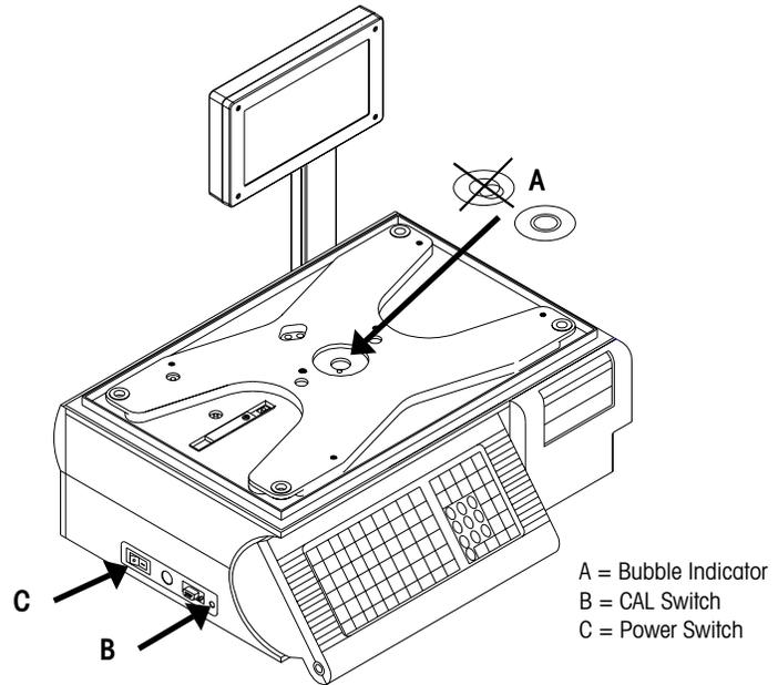
**Figure 2-4: Level Indicator, CAL Switch, and Power Switch**
