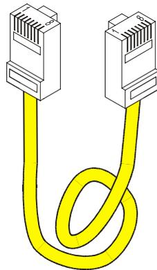
RJ-45 Connectors used on UTP 10BASE-T networks. METTLER TOLEDO® clients and the STEM use this connector.
