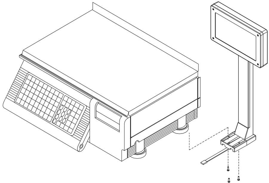
**Figure 2-2 Mounting the Display Tower (Except SSP)**
