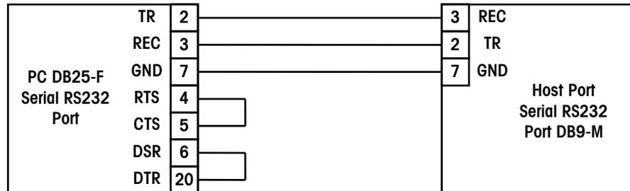
Model 8450 to PC RS232 Serial Port Wiring
