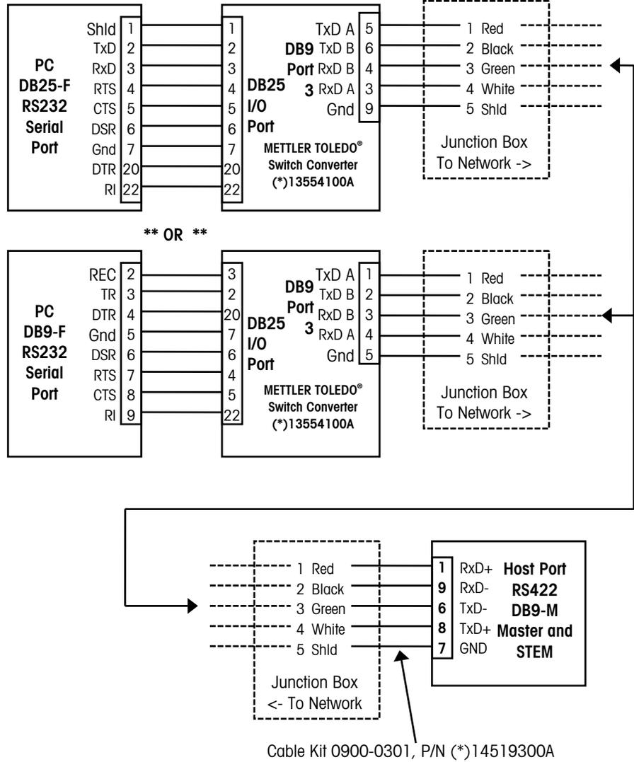
Model 8450 RS422 to METTLER TOLEDO® Converter Wiring
