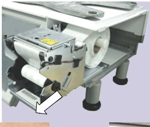
Slide the printer out for access to the printhead.
