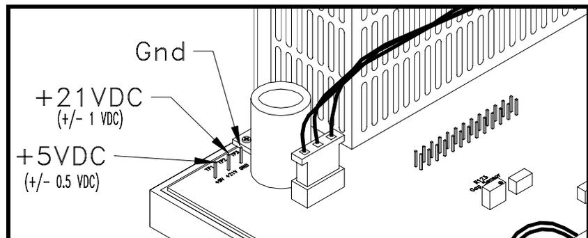
**Voltage Test Points on Main Logic PCB**
