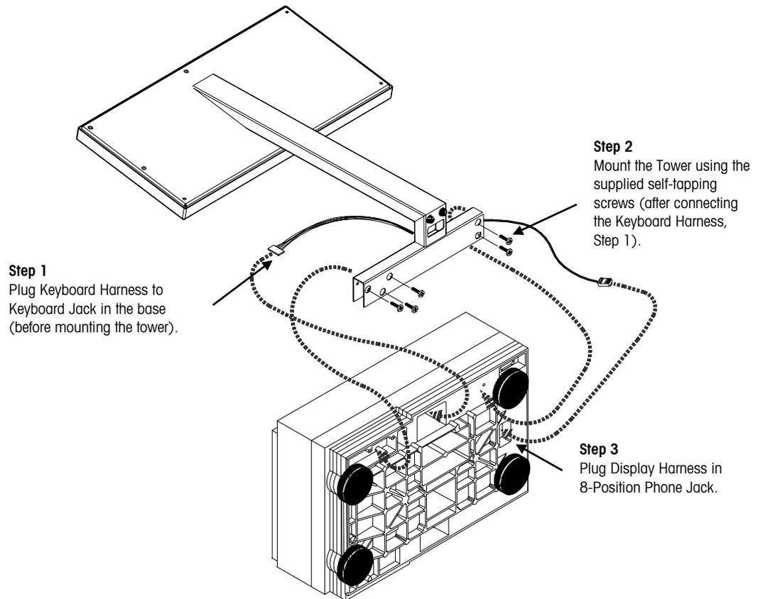
**Figure 2-5: SSP Tower Installation**
