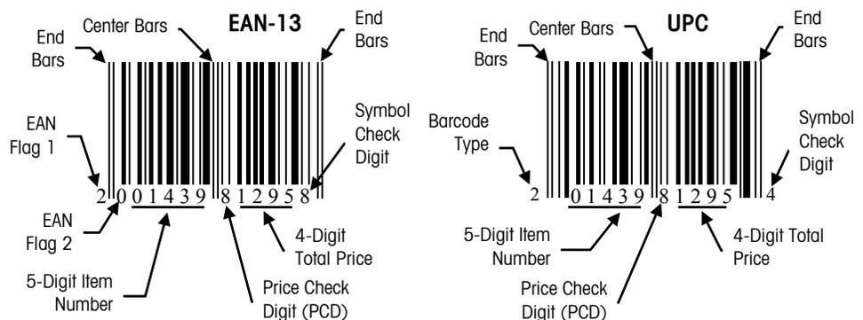
Figure 1-12: Barcode Symbols/Price Check Digit (PCD) Enabled
