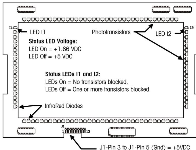
Touchpanel PCB Voltage Test Points
