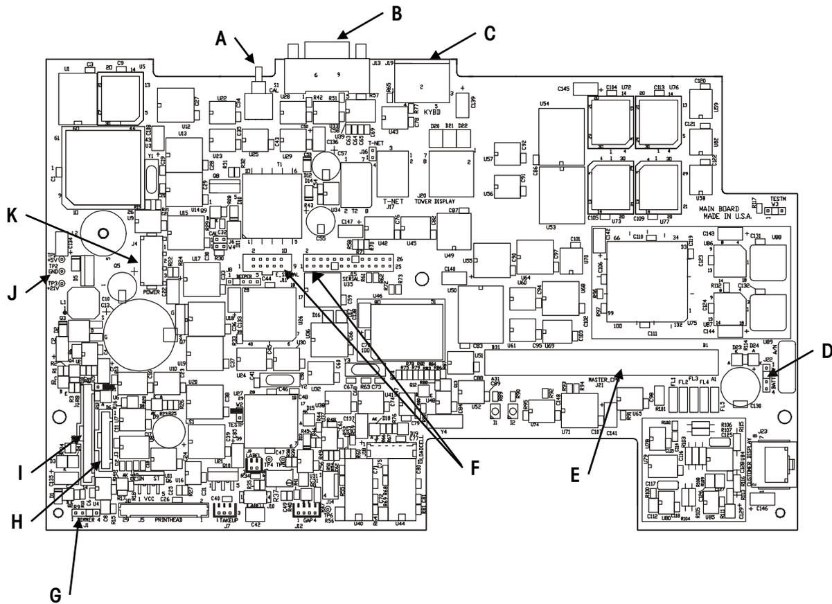
Figure 1-5: Main PCB Layout
