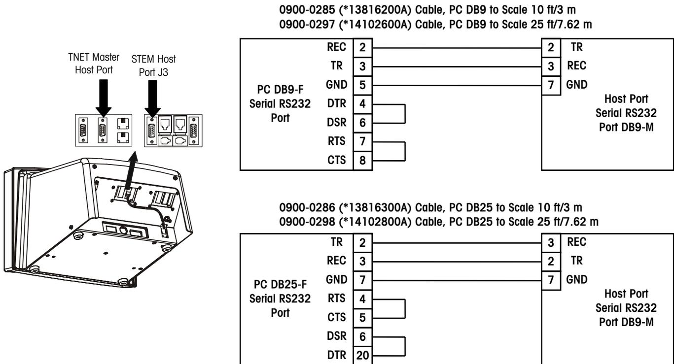
Figure 4-8: SmartTouch® Master to PC RS232 Serial Port Wiring
