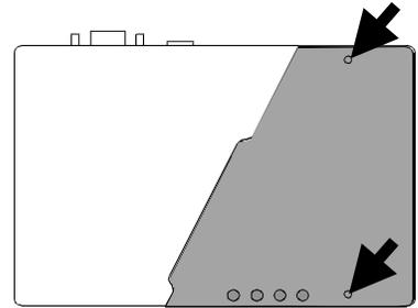
Next, slide the PCMCIA card out from the adapter. Disconnect the antenna leads from the card. Reconnect the antenna leads to the new radio card, and then slide the new radio card in the adapter. Push the card in until you can feel the card plug into the receptacle. Route the antenna leads out the top of the adapter and on top of the strain relief block so they are clamped in place when the cover is installed (see below).
