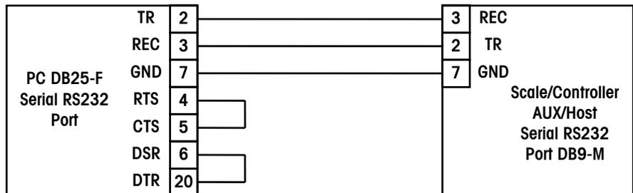
Figure 4-1: PC RS232 to Host/AUX Port Cables
