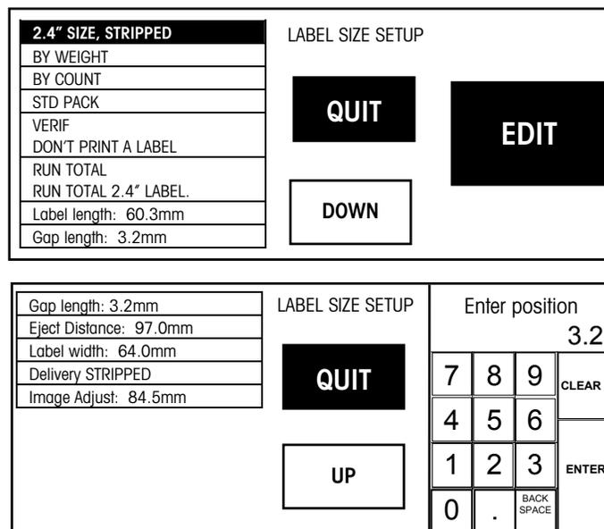
Figure 3-34: Setup Menu for a particular label size
