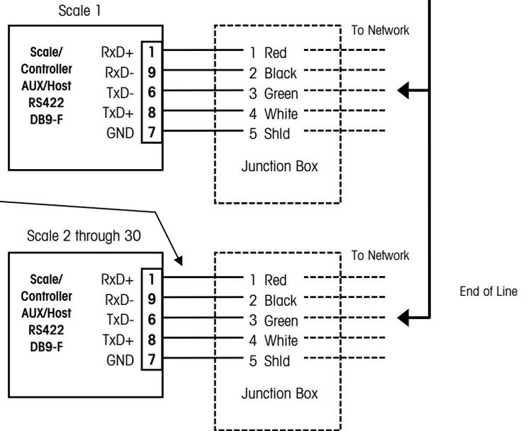
**Testing the RS422 Wiring**
