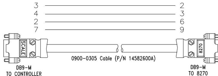
Figure 2-4: Scale Interface Cable
