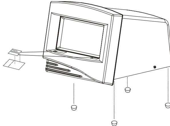
Figure 2-2: Installing Stick-On Feet and Capacity label
