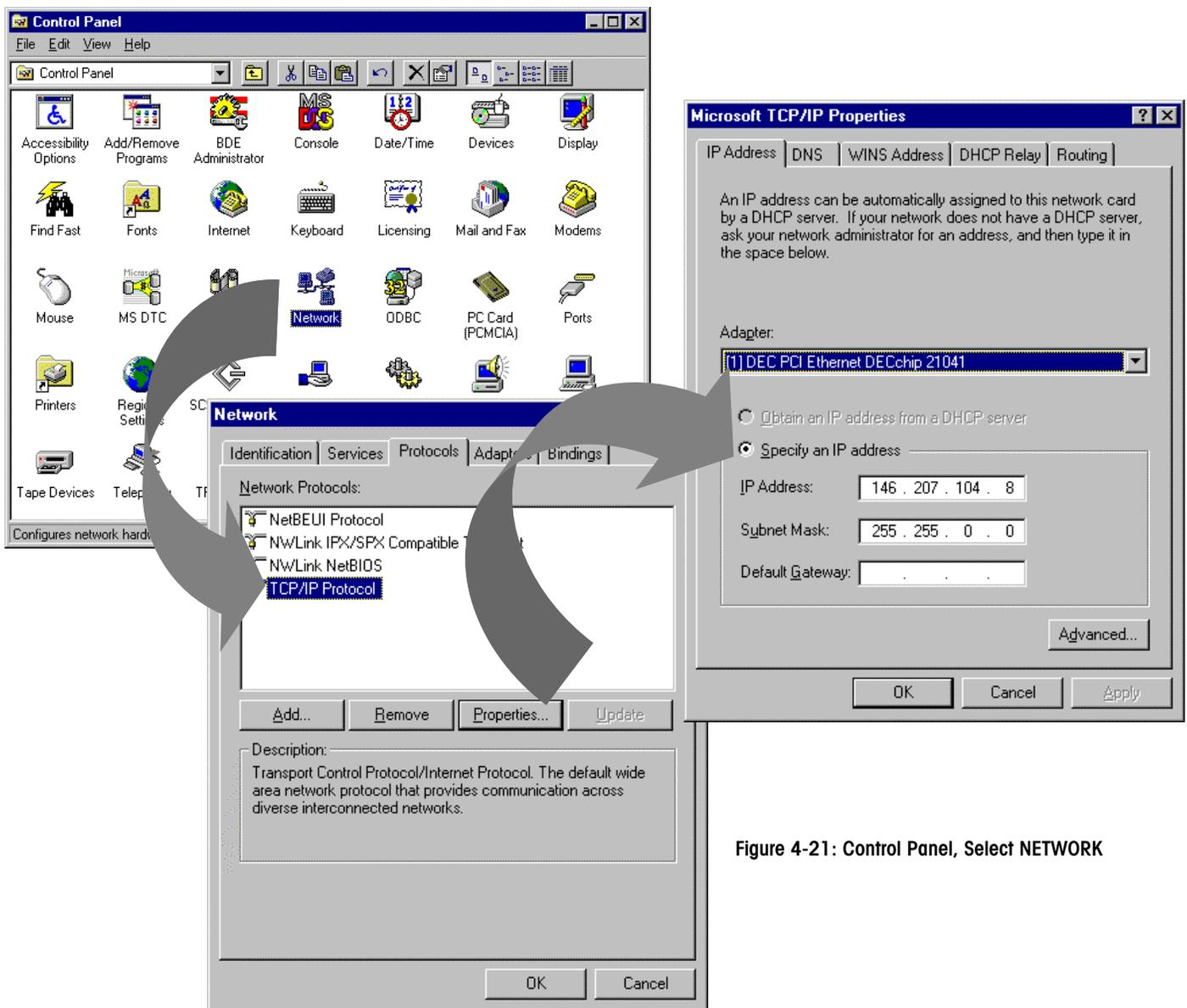
Figure 4-21: Control Panel, Select NETWORK
