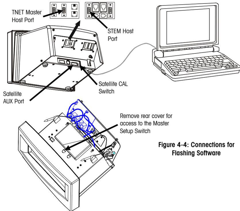
Figure 4-4: Connections for Flashing Software
