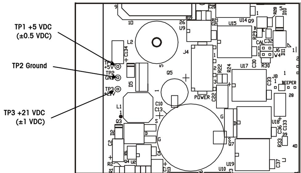
Voltage Test Points on the Main PCB
