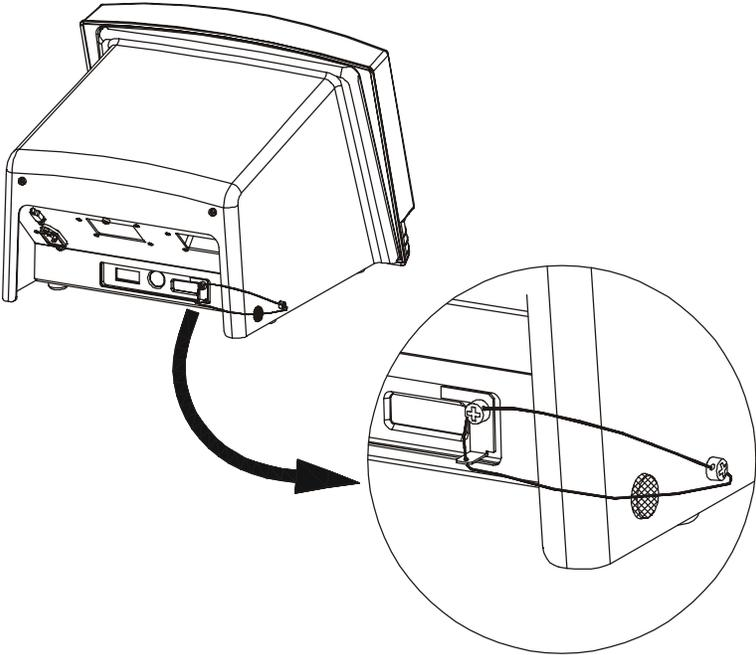
Figure 2-7: Sealing Screw and Bracket Installation
