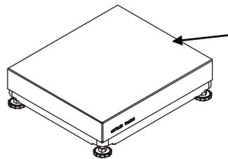
1. Empty the platter before continuing. Touch CALIBRATE, then touch ENTER to start calibration.
