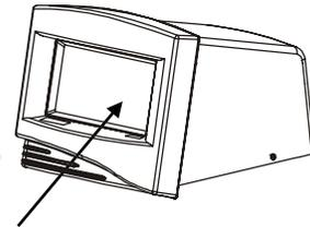
2. With the platter empty, touch CONTINUE to calibrate zero. The unit will count down from 15 to 0 while zero is set. Do not disturb the unit while it is setting zero.
