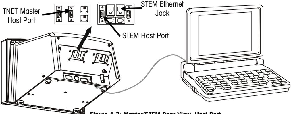
Figure 4-3: Master/STEM Rear View, Host Port
