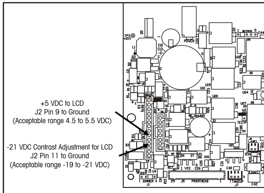
LCD Contrast/Voltage Test Points on Main PCB
