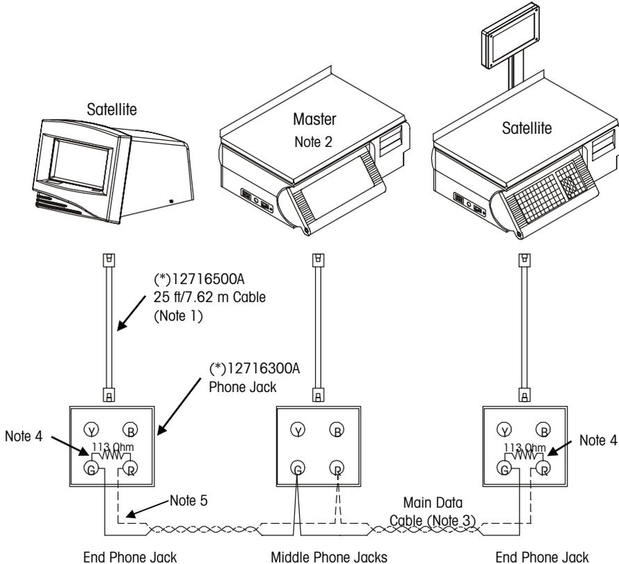
Figure 4-7: TNET Network Wiring
