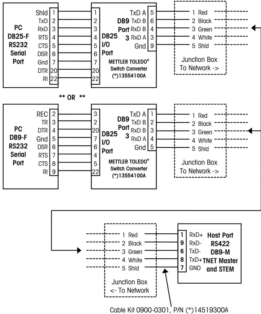
Figure 4-9: SmartTouch® Master RS422 to METTLER TOLEDO® Converter Wiring
