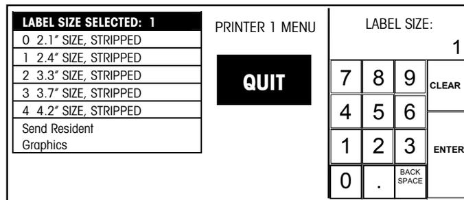
Figure 3-33: Menu Options for setting up Printer 1
