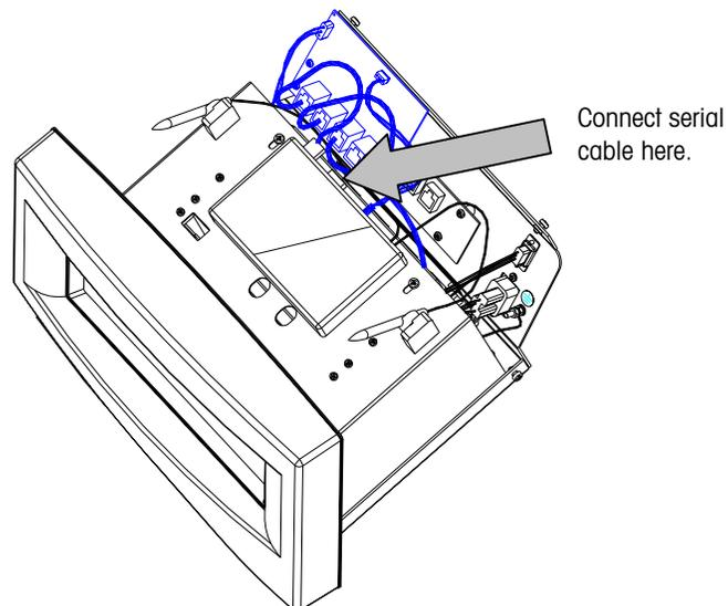
Connecting a Serial Cable to Mercury-PC Module
