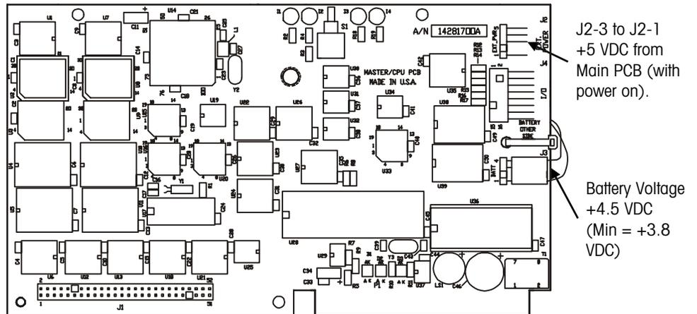
**Master CPU Voltage Test Points**
