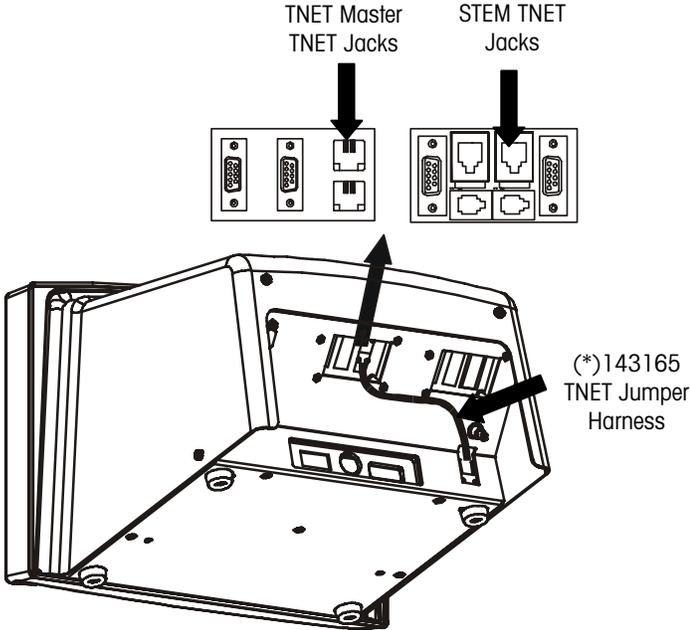
Figure 4-6: SmartTouch<sup>®</sup> Master TNET Connectors
