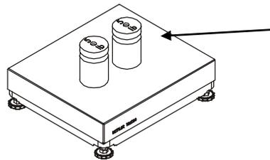
3. When zero has been set, add test weight to the platter. The minimum recommended weight is 20 lb/10 kg.
