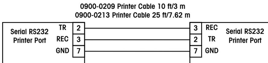
Figure 3-51: SmartTouch® Master to 88XX RS232 Printer Cable
