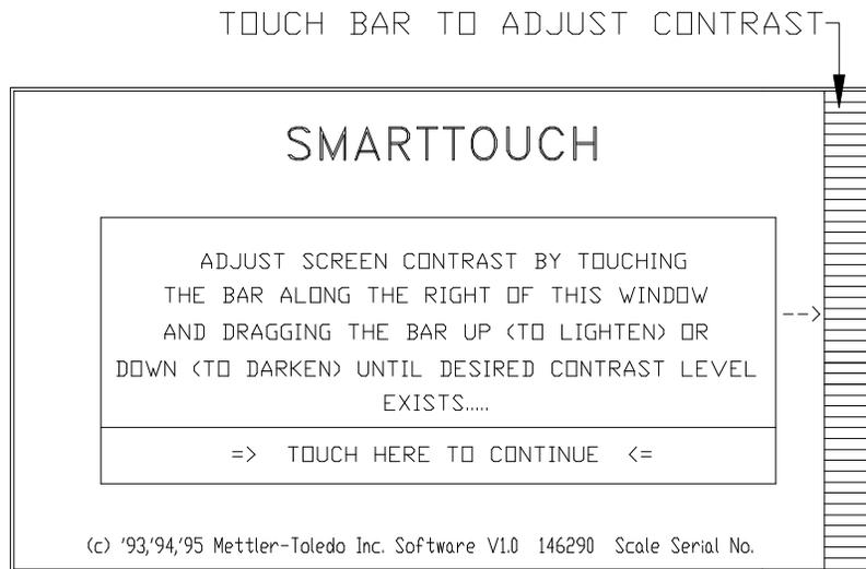
**Figure 2.1 - Adjust Contrast Screen**
