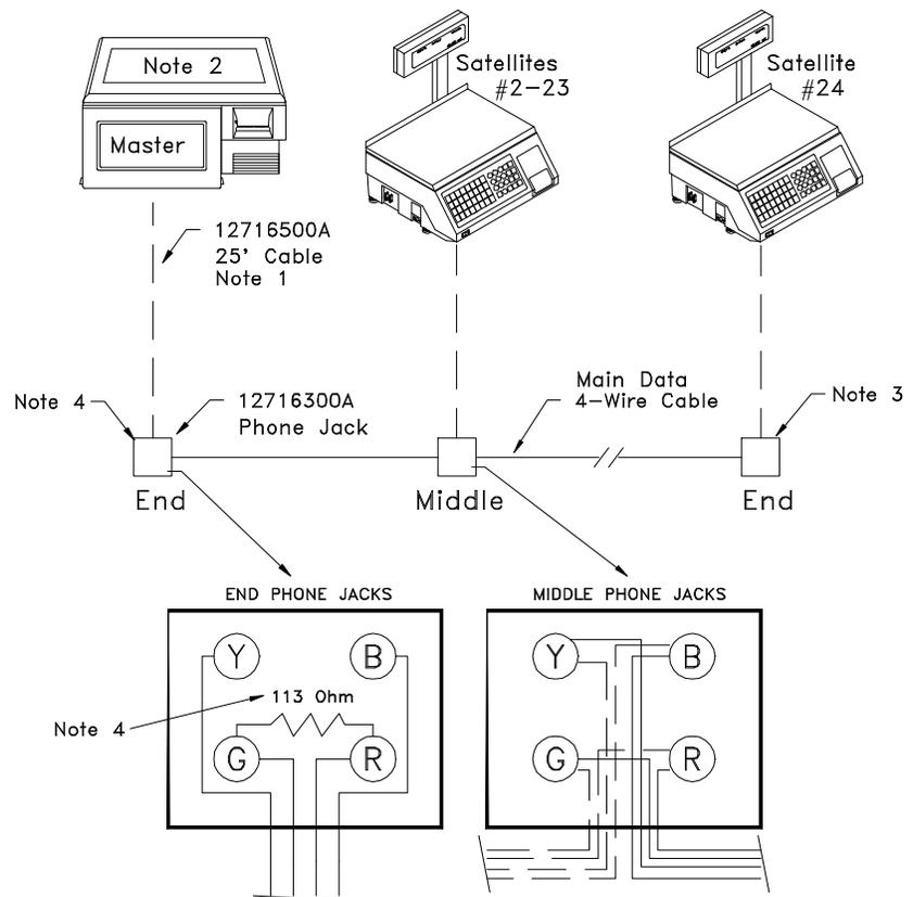
**Figure 3.3 Master/Satellite TNET Wiring**
