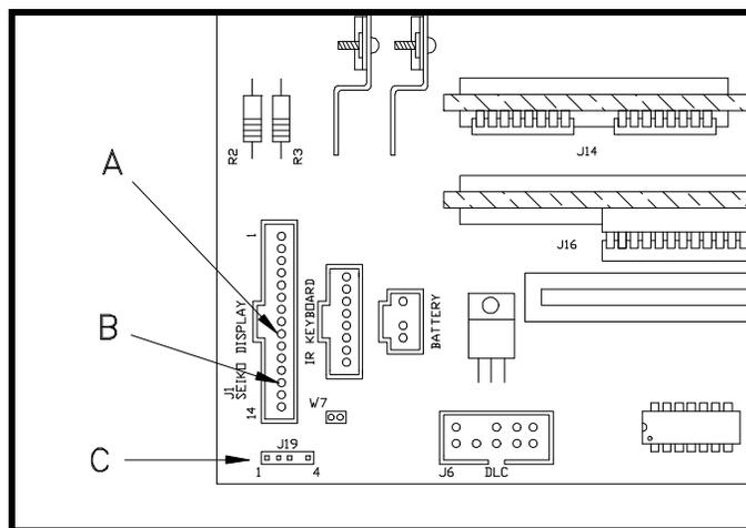
**Figure 4.7 LCD/Backlight Test Points on Mother PCB**
