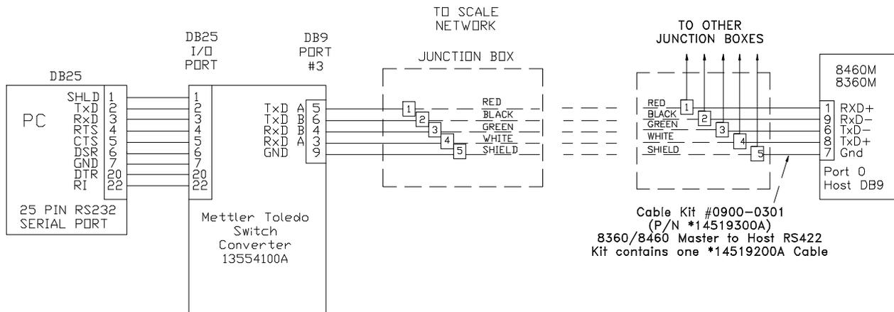
Figure 2.20 - Master RS422 Host Interface Wiring
