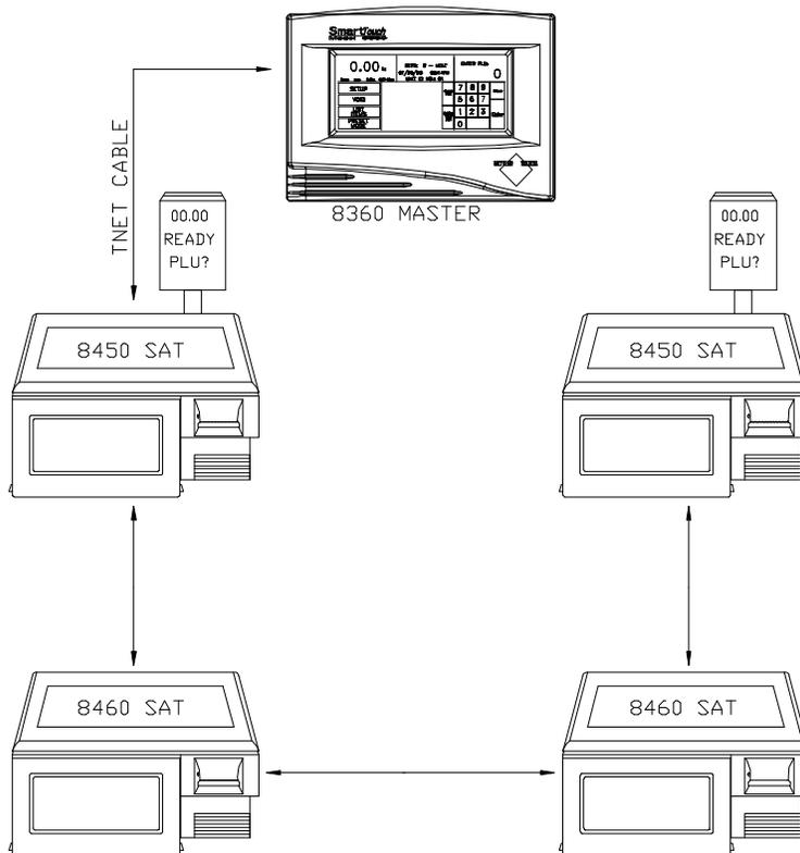
Figure 1.2 - Master/Satellite Network (TNET)
