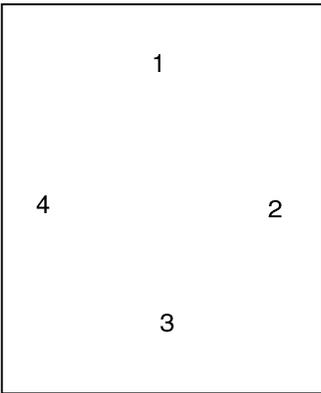
Figure 4-c: NIST H-44 Shift Test Position
