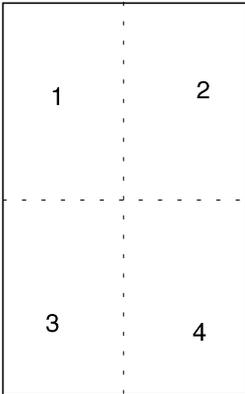
Figure 4-d: OIML R7C Shift Test Points
