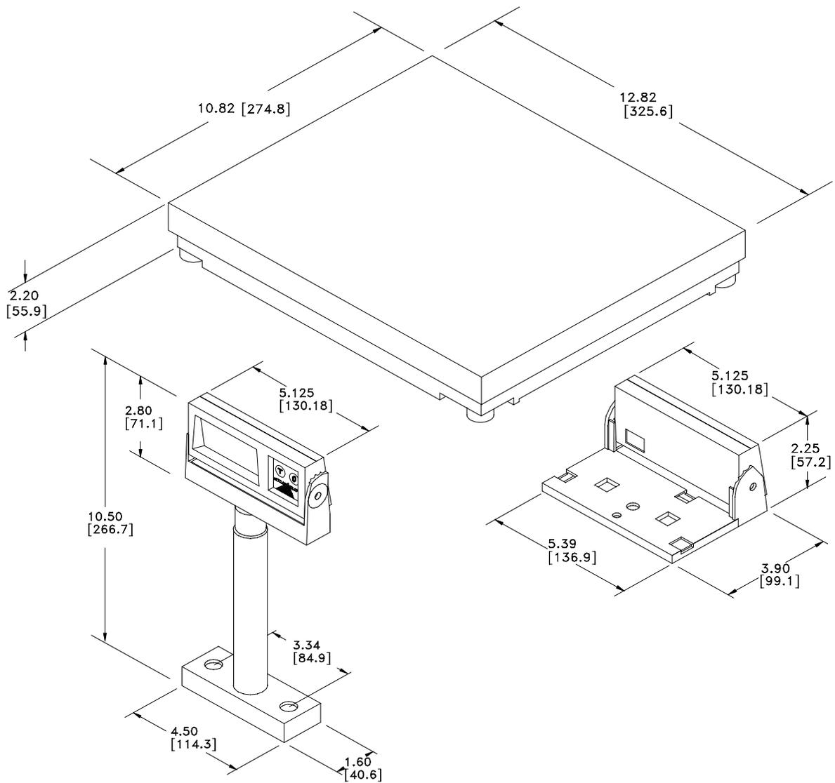
Figure 2-a: 8217 Dimensions (Shown with Optional Displays)
