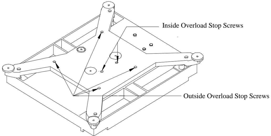
Figure 4-e: Overload Stop Adjustment
