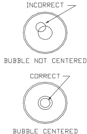
**Figure 4-a: Leveling Bubble**
