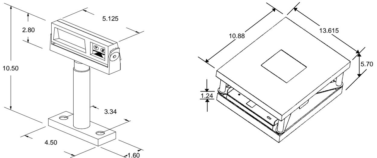
Figure 13-a: Dimensions (Shown with Remote Display)
