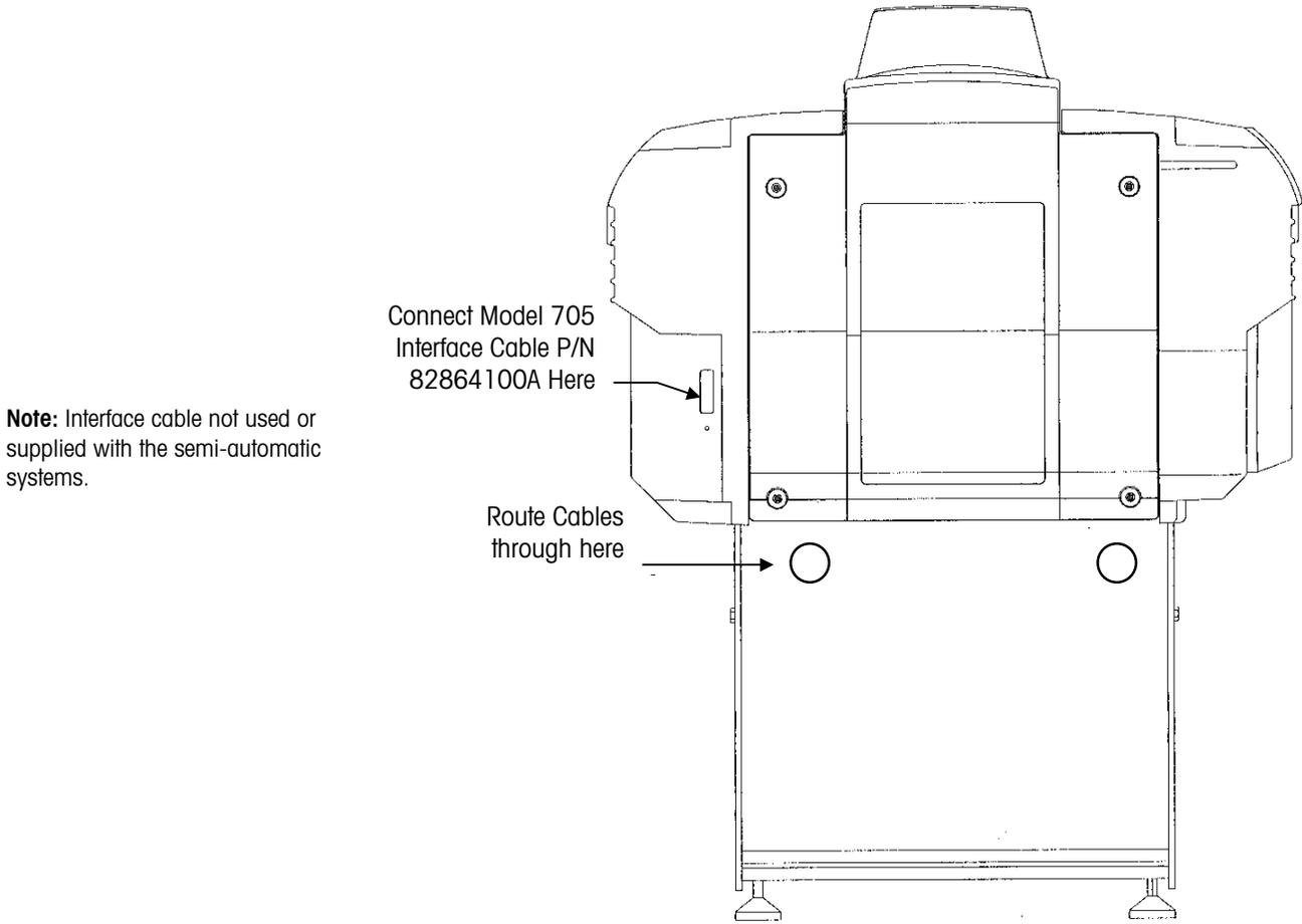
**Note:** Interface cable not used or supplied with the semi-automatic systems.
