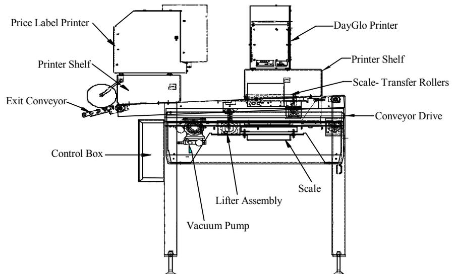
Figure 1-1 Model 705 Labeler Components
