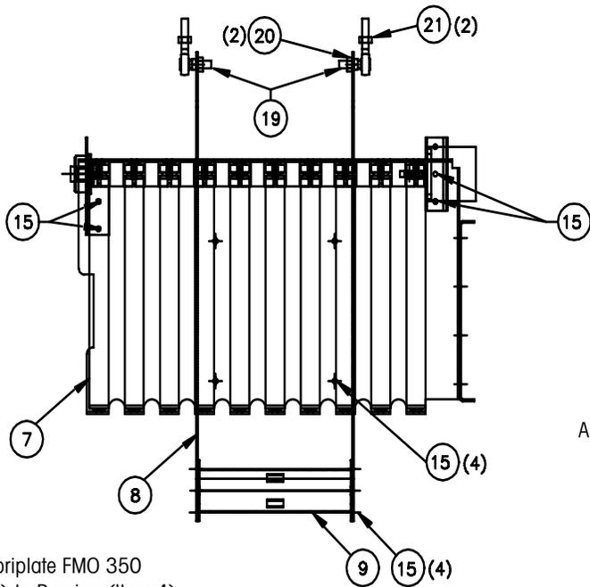
Apply Lubriplate FMO 350 (Item 22) to both roller bearings.
