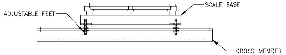
Figure 5-2: Model 8270 Scale Base and Support
