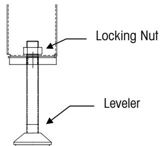
Figure 4-2: Model 705 Labeler Leveler
