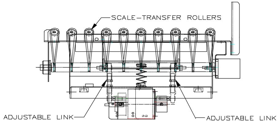
Figure 5-4: Lifter Assembly
