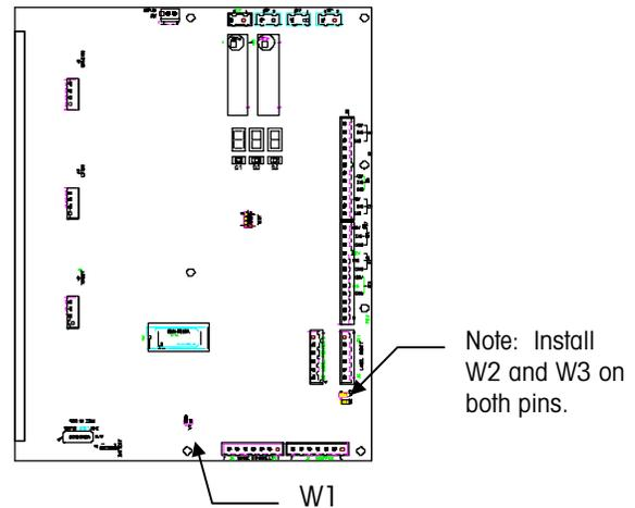
Figure 4-9: Circuit Board Jumper Settings
