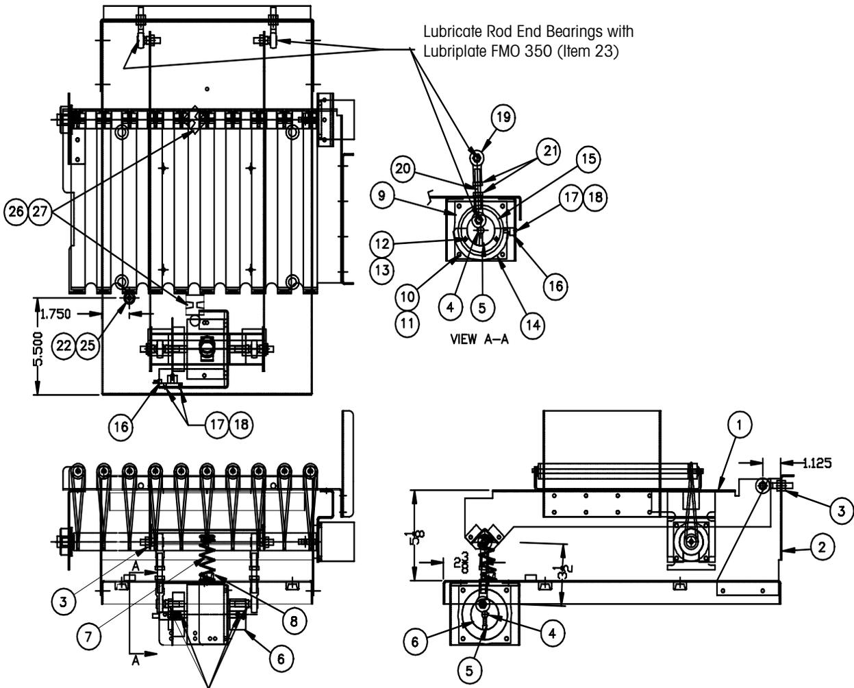
Use Loctite 242 (Blue) (Item 24) on Rod End Thread and Set Screws in Lifter Cam (Item 6)
