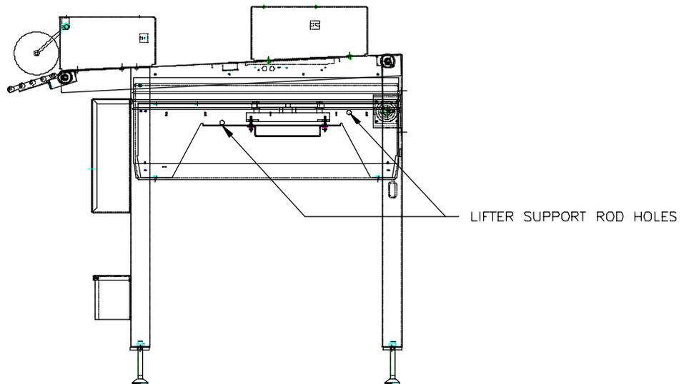
**Figure 5-1: Lifter Support Rod Hole Location**
