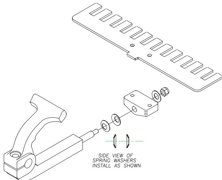
**Figure 7-18: Center Clamp Film Gripper**
