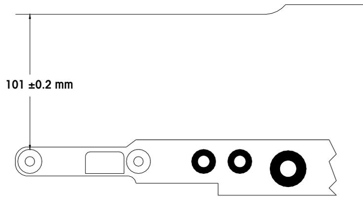
Figure 7-43: Sealing Belt Position Measurement
