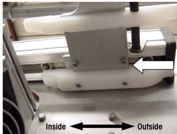
When reassembling the linear actuator, make sure the orientation is correct. When installed correctly, the mounting plate is flush towards the outside of the machine and will stick out slightly toward the inside of the machine.
