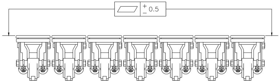
**Figure 7-29: Side Clamps Horizontal Plane Check**
