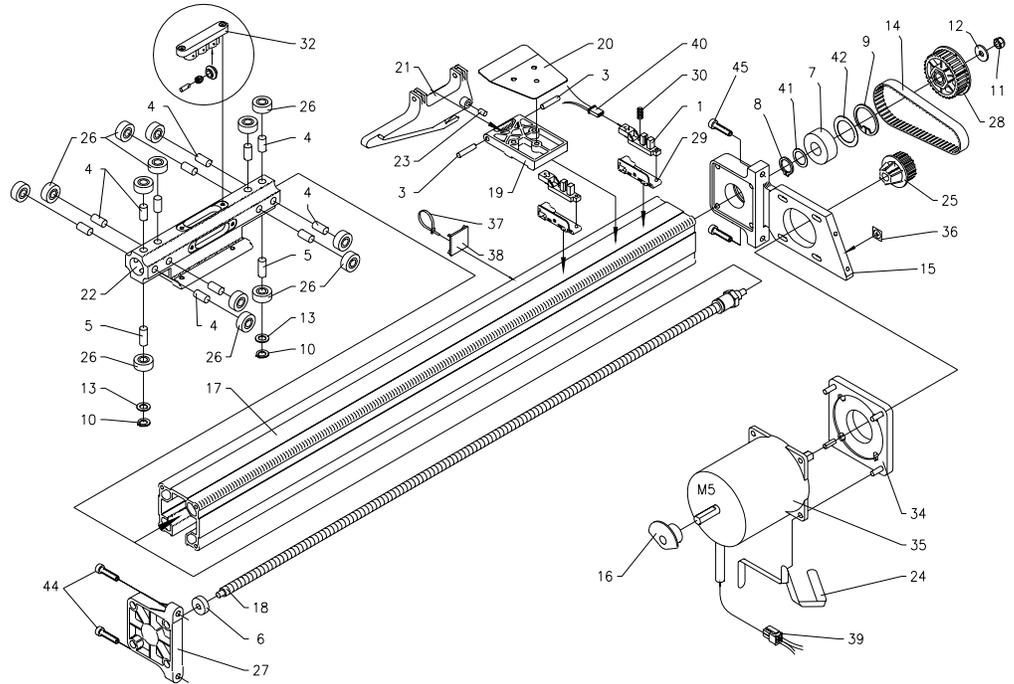
Figure 7-21: Center Clamp Linear Actuator Service
