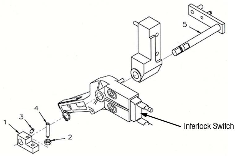
Figure 7-6: Infeed Door Interlock Switch
