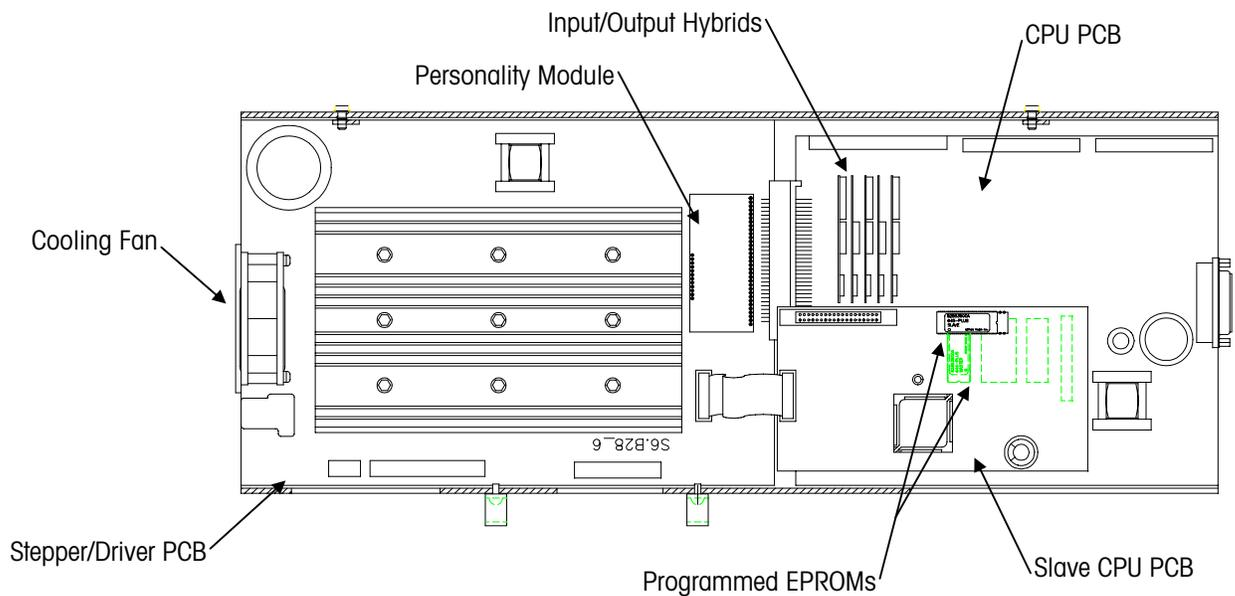
**Figure 7-48: Electronics Rack**
