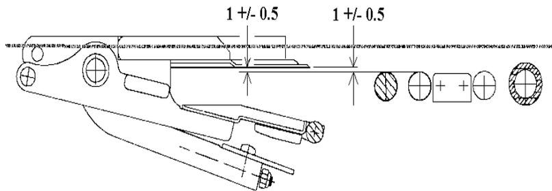
**Figure 7-23: Clearance Between The Clamp and Exit Rollers**
