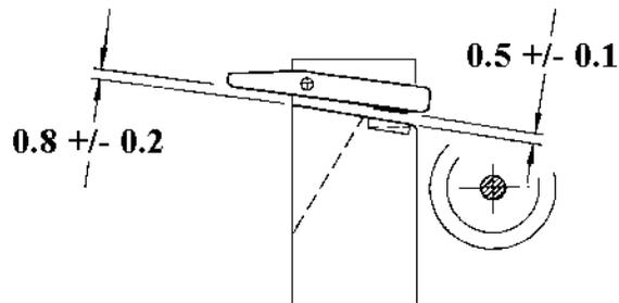
Figure 7-37: Position of the Distributor Clamp Plate (Toothed Side)
