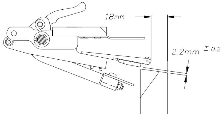
Figure 7-25: Film Clamp Clearance at the Distributor
