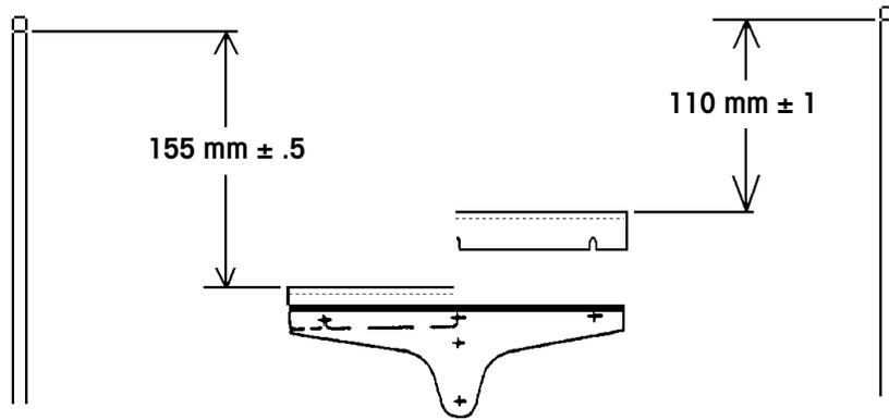
Figure 6-5: Cutter Channel Position Test
