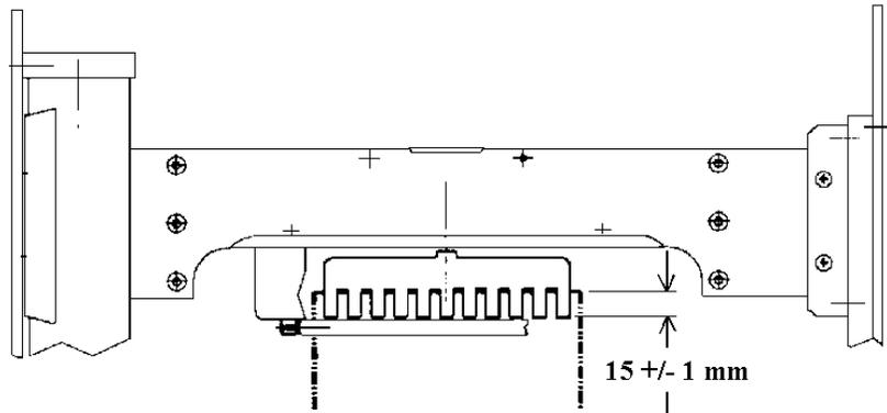
Figure 7-45: Checking the Film in the Center Clamp
