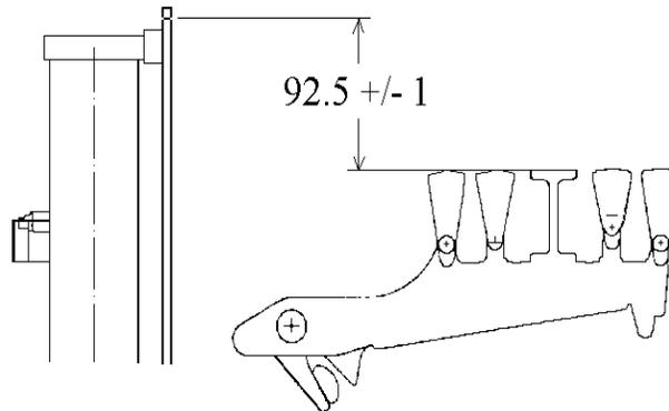
Figure 7-13: Lifter Stroke Measurement
