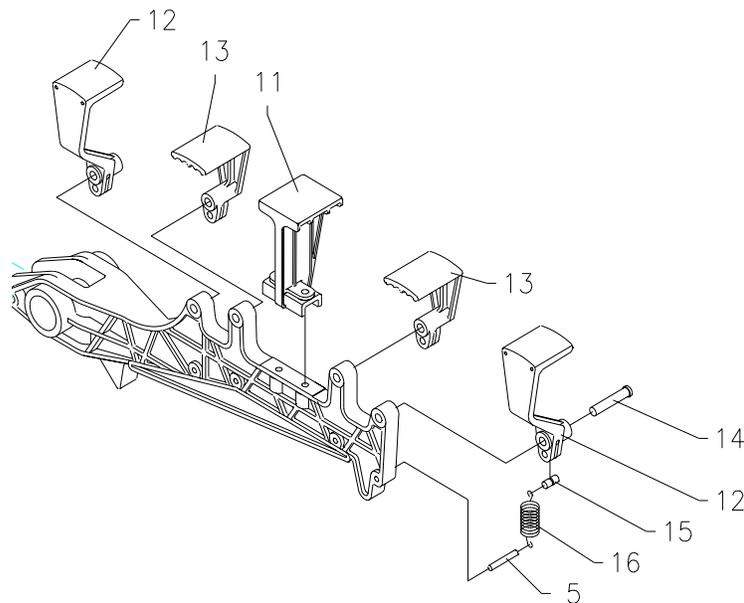
**Figure 7-8: Lifter Support Replacement**
