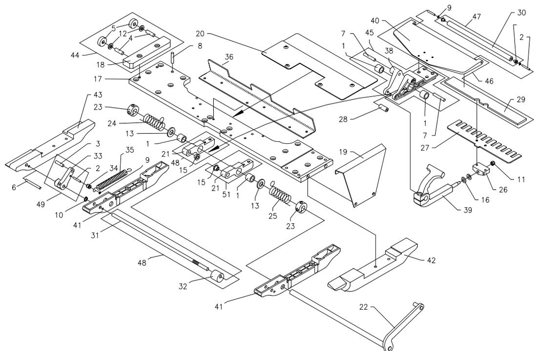
Figure 7-19: Film Gripper Mounting Lever Replacement
