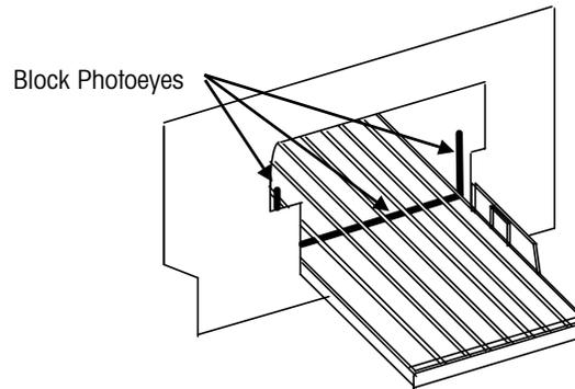
**Figure 6-2: Photoeye Test**
