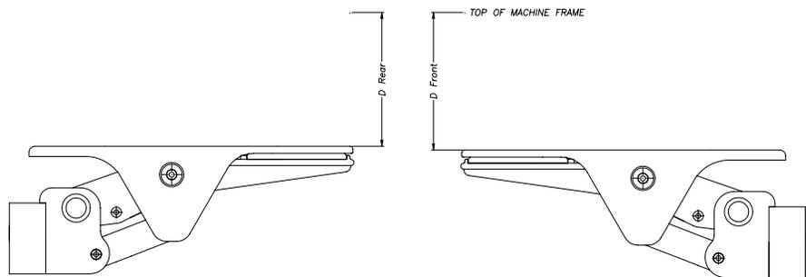
**Figure 7-30: Front to Rear Side Clamp Alignment**
