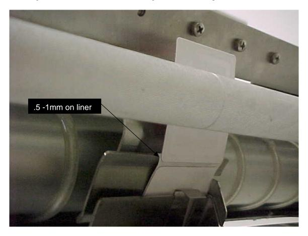
The leaf spring located on the label feed has an adjusting screw and locknut. The purpose of this spring is to hold the labels against the side of the stripper bar so they are released at the optimum angle for pick up. Create just enough spring tension to hold the labels against the label stock against the stripper bar. Excessive tension will cause excessive drag and will delay the issuing of the labels.
