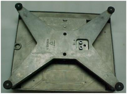
On 706 Autolabelers with serial number date codes prior to EB, it is necessary to replace the 4 screws that attach the scale platter to the scale conveyor with 4 M4x16mm screws P/N 82715500A and 4 spacers P/N 83140700A to maintain the proper position of the platter on the new style spider.
