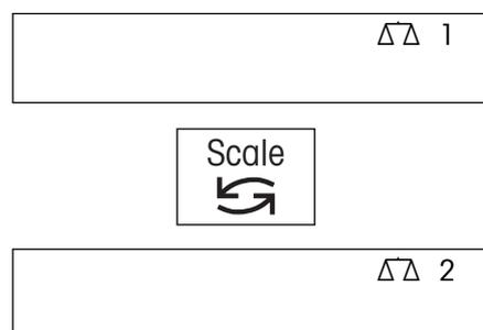
The scale symbol in the upper right-hand corner of the display indicates which scale is currently active ("ΔΔ 1" = Viper scale, "ΔΔ 2" = second scale).
