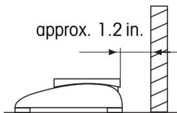
If the **power cable** is damaged, the scale must not be used. Check the cable regularly and ensure there is a clearance of approx. 3 cm (1.2 inches) behind the scale so the cable is not excessively kinked.
