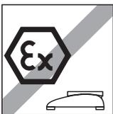
Do not use the scale in **hazardous environments** (unless it is specially marked for this purpose).
