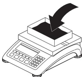
Place the weighing sample on the weighing pan ...
