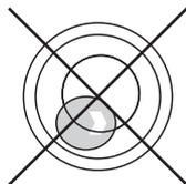
Adjust the scale horizontally by turning the leveling feet. If there is a level indicator, the air bubble must lie inside the inner circle.
