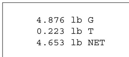
Pressing the «**Print**» key transmits the current weighing result via the interface to the peripheral device (printer, computer). At the factory the standard interface is configured for connection of a printer. Refer to Section 4.7 for information about configuring the interface(s).
