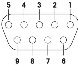
Standard Viper scales are fitted with one voltage interface according to EIA RS-232C/DIN 66020 (CCITT V24/V.28, maximum cable length 50 ft/15 m). As an option, Viper scales are also available with 2 interfaces. The corresponding interface boards replace the standard interface. An analog interface is also available instead of an RS232C interface. All interfaces have a 9-pin sub-D socket (female).
