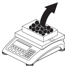
Remove the reference number of pieces from the container and then press the «**Sample**» key.
