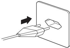
Before connecting the power supply, check that the voltage printed on the right side of the scale, or on the AC adapter, is the same as the local power supply voltage.
