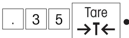
Enter the known tare weight in the current weighing unit on the numeric keypad and confirm with the «**Tare**» key. If the entry is incorrect, it can be deleted digit-by-digit with the «**C**» key.
