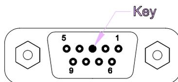
Figure 6-1 DigiTOL® Load Cell Connector
