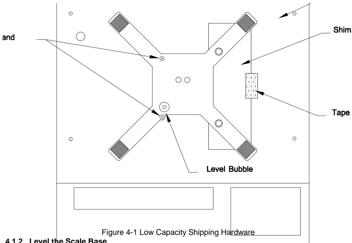
Level the scale by turning the adjustable feet on the bottom of the scale base until the level indicator is correct. The feet must be adjusted so the scale does not rock. Carefully tighten the lock nut at each adjustable foot. Refer to Figure 4-2.
