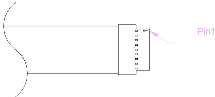
Figure 7-6 Keyboard Connector Pin 1
