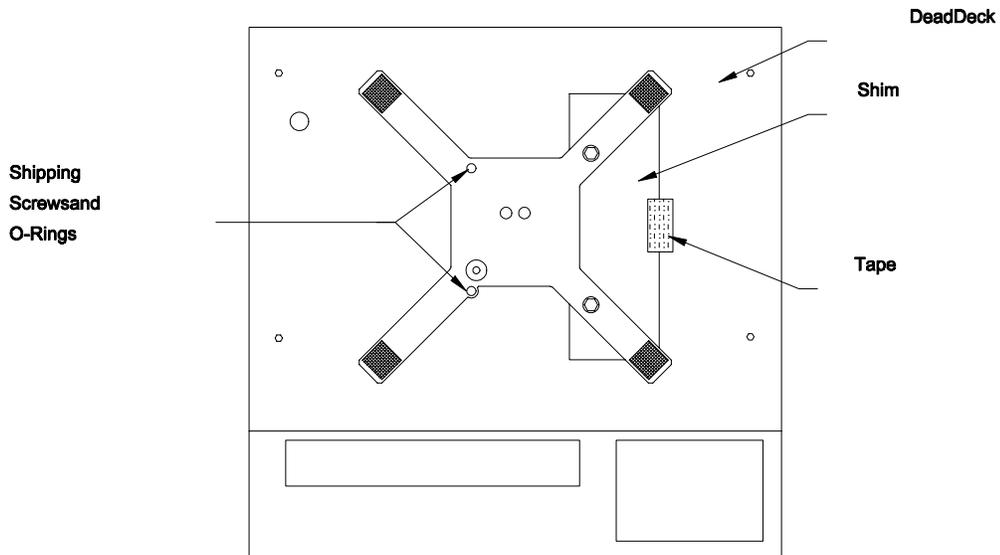
Figure 7-2 Low Capacity Shipping Hardware
