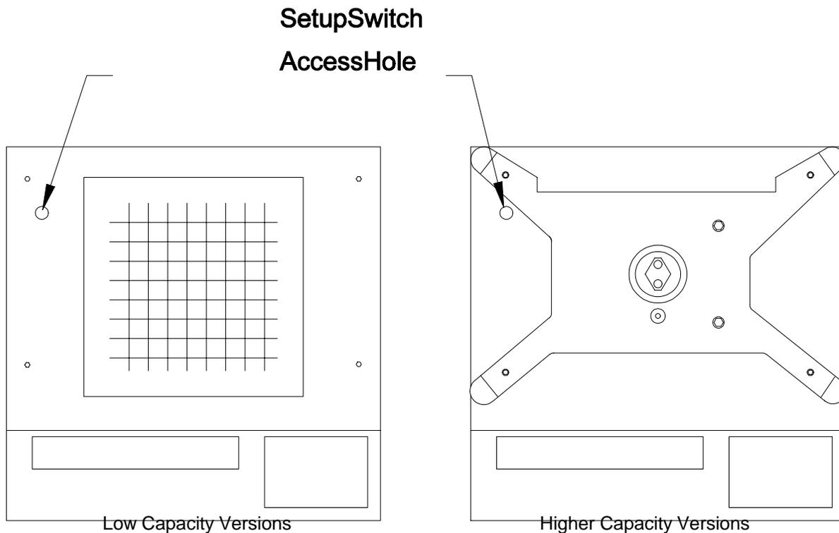
Figure 4-3 Setup Switch Access Hole
