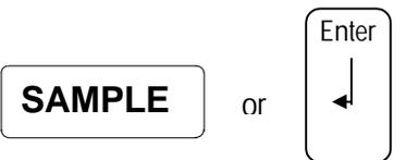
Press the **SAMPLE** key to acknowledge the placement of sample pieces.
