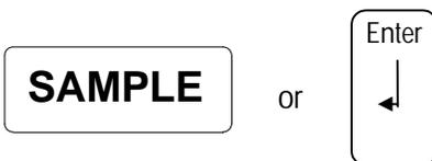
Press the **SAMPLE** key to acknowledge the placement of sample pieces on the weighing surface.
