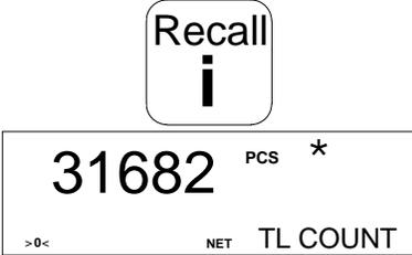
Pressing the **RECALL** key again will retrieve the next data field from memory. Each time the **RECALL** key is pressed, the next field in sequence will be recalled.
