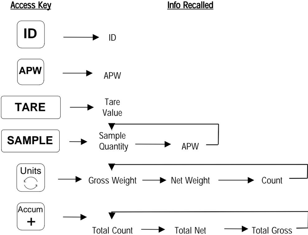
To recall any of these fields or "groups," press the **RECALL** key then the access key shown in the chart above. The display will show the field in the first column on the display. For keys which contain data in either the second or third recall column, repeated pressing of the access key will toggle the display through each of these fields.
