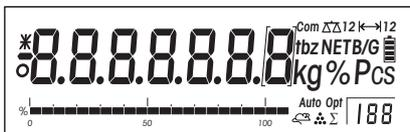
After the last key has been checked the scale lights up all segments of the display. Make sure all segments are visible. Pressing any key aborts the display test.
