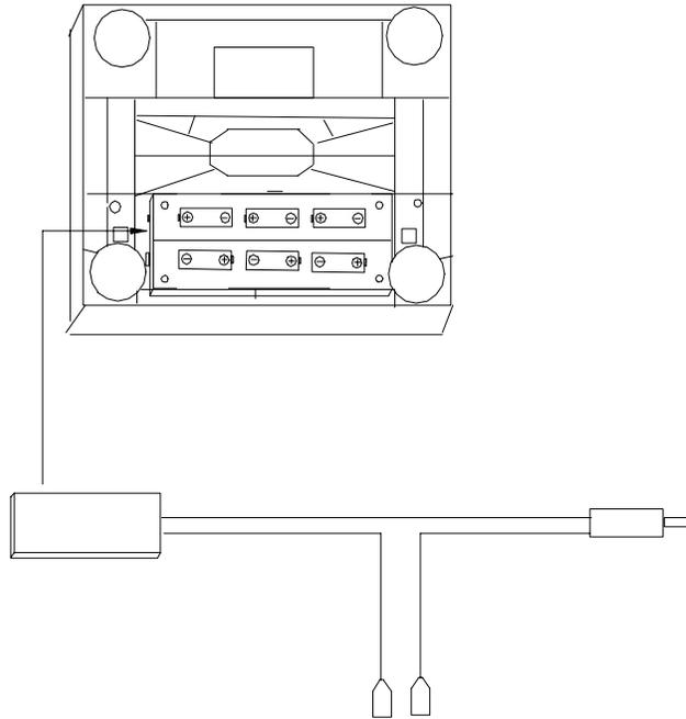
4. Insert the on/off rocker switch (P/N 14262400A) into the switch hole of the battery cover (P/N 14545200A) noting the orientation of the switch.
