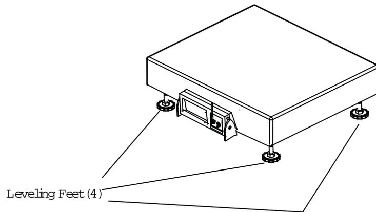
Figure 2-a: PS and PS6L Leveling Feet
