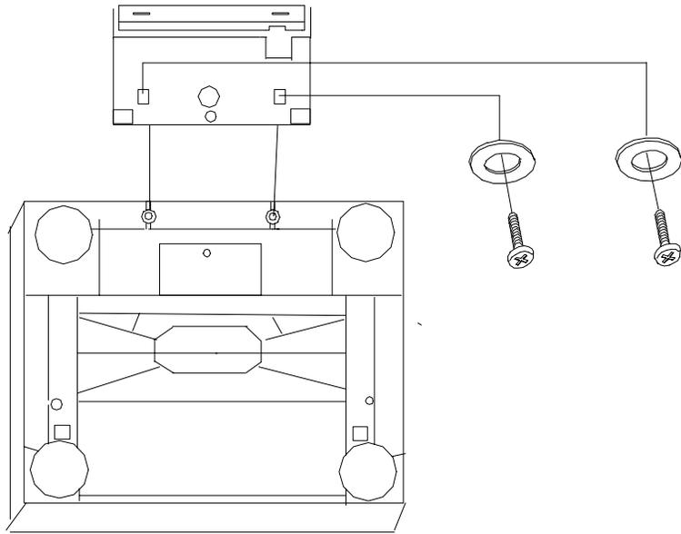
2. Install the display interface harness from the display as shown. Insert the display interface harness into the PCB as shown. Make sure to route the cable as shown to prevent damage to the cable.
