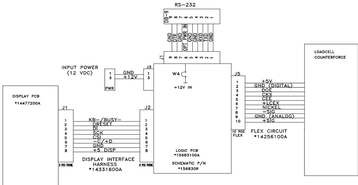
Figure 1-c: PS Electronic Interface Diagram
