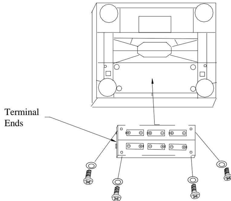
3. Attach the harness assembly (P/N 14544600A) to the battery holder.
