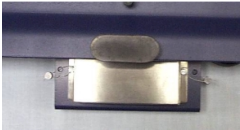
Figure 2-g: Wire Seal Installation
