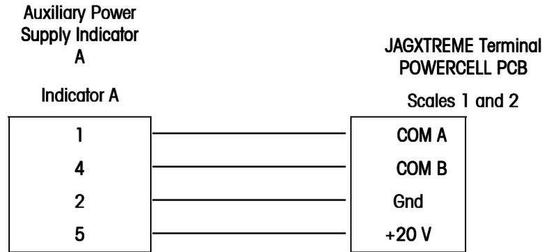
If a second JAGXTREME terminal exists, the interface cable between the second terminal and the Auxiliary Power Supply would be wired the same. However, the interface cable would plug into the Auxiliary Power Supply at INDICATOR B. The W1 jumper on the Auxiliary Power Supply **must not** be shorting the two pins together.
