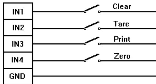
Figure 2-g: Input Wiring Example
