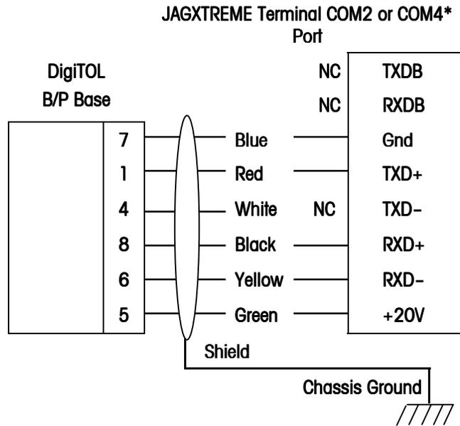
\*When interfacing a DigiTOL or UltraRes base to COM4 (available on the optional Multifunction PCB), W2 must be set for 20V. Refer to the section entitled JAGXTREME Terminal Jumper and Switch Settings in this chapter.
