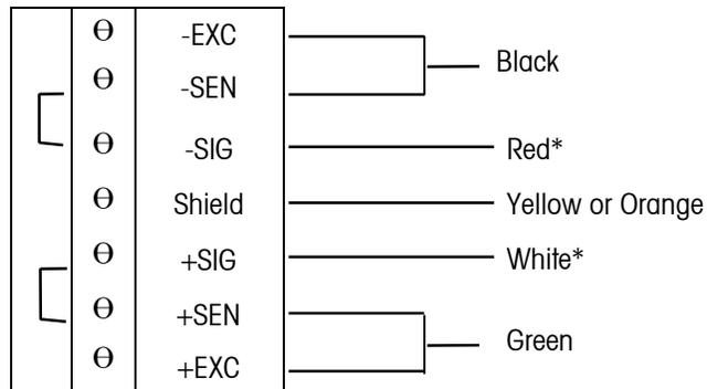
\* If an increase in load results in a decrease in weight display, reverse the signal wires (+SIG and -SIG).
