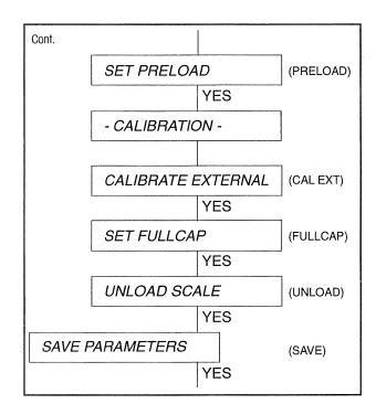
Unload weighing platform. Attach special external fittings or preloads if desired by customer.
