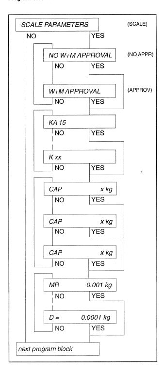
In this program block the parameters specific to the weighing platform, namely admissibility for certification (approval), maximum capacity, range and scale interval are entered.
