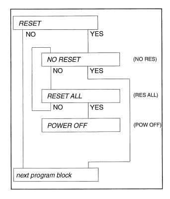
In this program block the parameters specific to the weighing platform, namely admissibility for certification (approval), maximum capacity, range and scale interval are reset to the factory setting.
