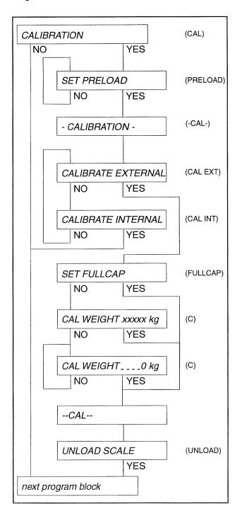
This program block is used for calibration of the scale.
