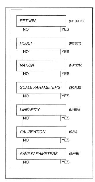
The first program block RETURN allows the service mode to be quit without a change in the set parameters and the ident code counter.
