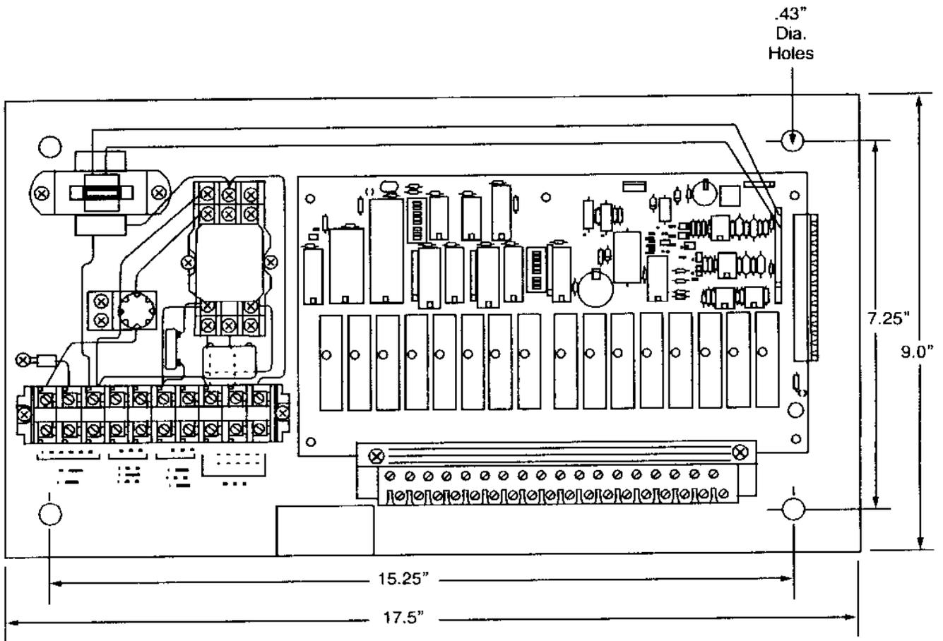
Figure 1.5 Panel Mount SmartLink Remote I/O PCB
