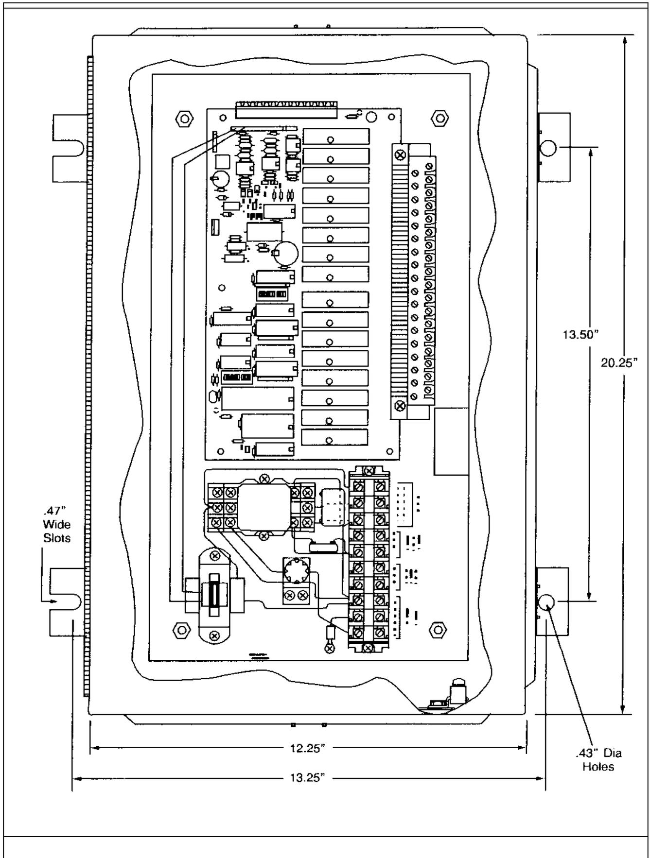
Figure 1.4 Wall Mount SmartLink Remote I/O Box
