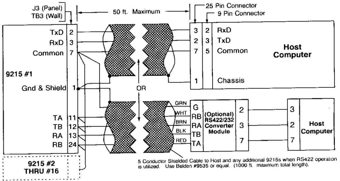
**Figure 3.2 9215 Interface Connection to Host Computer**
