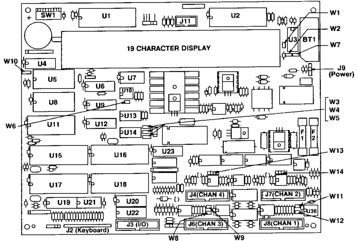
**Figure 1.2 TSM-300 PCB Identifications**
