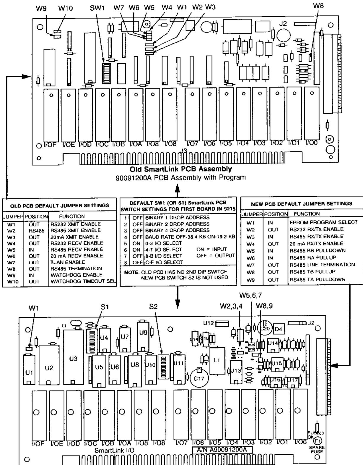
Figure 1.3 SmartLink PCB Identifications
