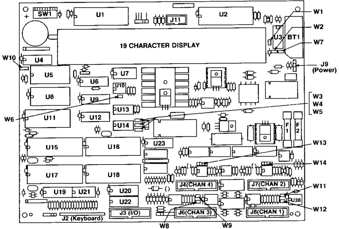
**Figure 3.6 TSM-300 PCB Identifications**
