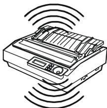
QUIET lets you turn the quiet mode on and off. In quiet mode, the print speed slows down by about 10% in all modes to decrease the amount of noise that is generated. You can select *On* to turn the quiet mode on or *Off* to turn the mode off.
