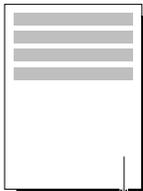
AUTO FF lets you turn the automatic form feed mode on and off. In the automatic form feed mode, the printer skips over the perforations of pin-feed paper by setting the top and bottom margins to one-half inch. You can select *On* to turn the automatic form feed mode on; or *Off* to turn the mode off. For the automatic form feed mode to work correctly, the LENGTH (page length) parameter must be set to the correct page length.
