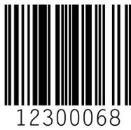
A bar code symbol consists of parallel lines and spaces of varying widths or heights. The bar code symbology describes unambiguous rules for encoding data into the bars and spaces.
