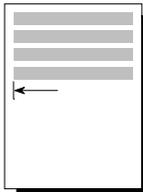
AUTO CR lets you turn the automatic carriage return mode on and off. In the automatic carriage return mode, the printer performs a carriage return/line feed for each line feed code it receives. You can select *On* to turn the automatic carriage return mode on; or *Off* to turn the mode off.
