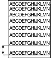
LPI lets you specify how many lines to print per inch. You can select 3, 4, 6, 8 or 12 lines per inch. If the current setting is *Other*, then your software application has set the number of lines per inch to some non-standard value.
