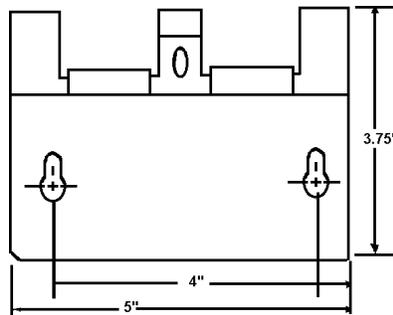
2. Mounting hole dimensions for wall mounting the stainless steel enclosure.
