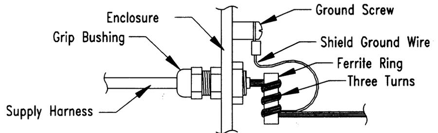
Figure 2-8 Ferrite Ring for Desk Enclosure with AC Power Supply
