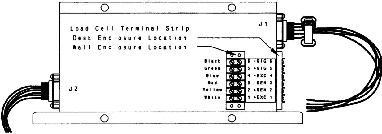
J1—Analog Load Cell Input from Terminal Strip
