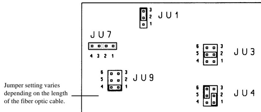
Figure 2-13 Jumper Selection for 20 mA Current Loop Active Transmit, Passive Receive
