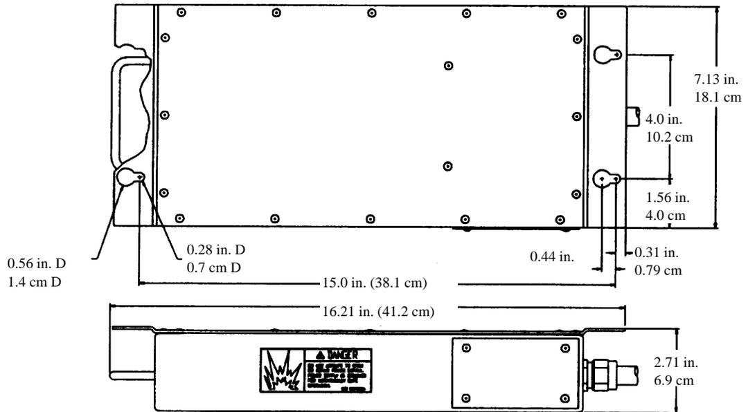
Figure 1-3 8525 10 AH Battery Pack Dimensions
