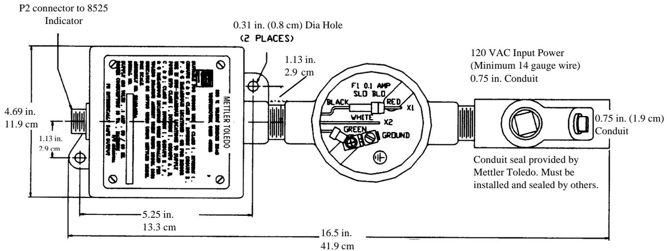
Figure 1-5 120 Volt AC Power Supply Dimensions
