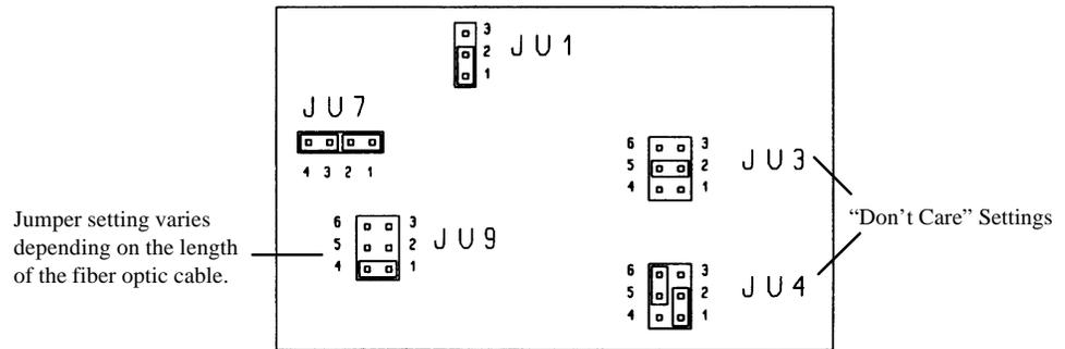
Figure 2-14 Converter Jumper Selection for RS-232 Printer and Computer Interfacing
