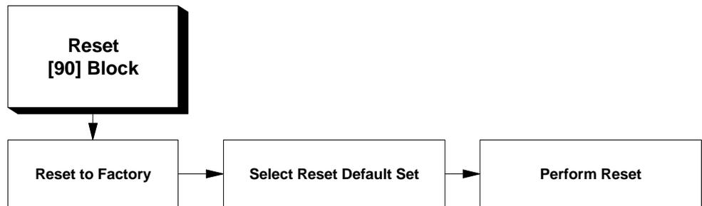
To reset the 8525 setup parameters to factory default settings:
