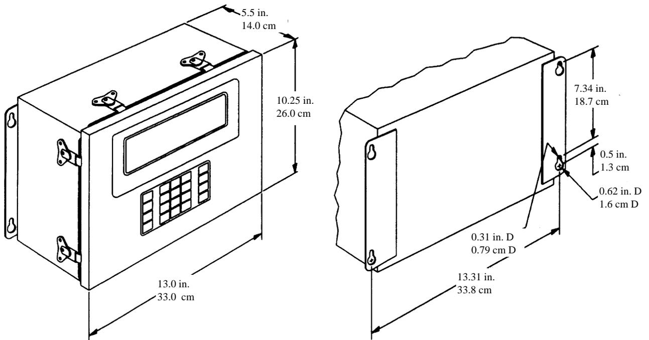
Figure 1-2 8525 Wall Enclosure Dimensions
