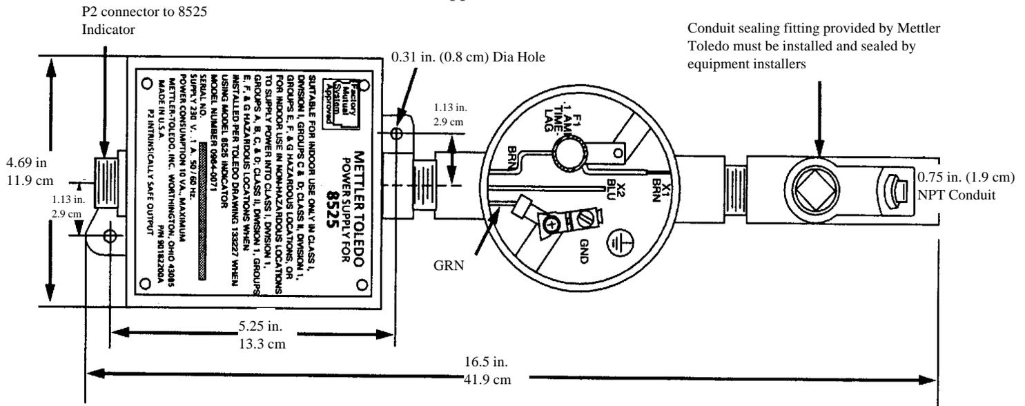
Figure 1-6 230 Volt AC Power Supply Dimensions
