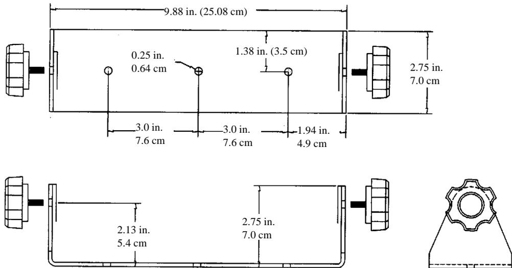
Figure 2-15 Desk Enclosure, Mounting Bracket Dimensions
