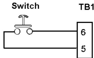
**Serial I/O Remote Pushbutton "Contact Closure" Input**
