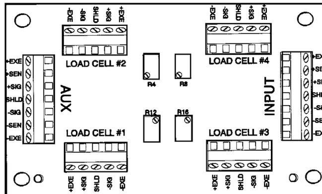
**Figure 6-13 - Analog J-Box PCB**
