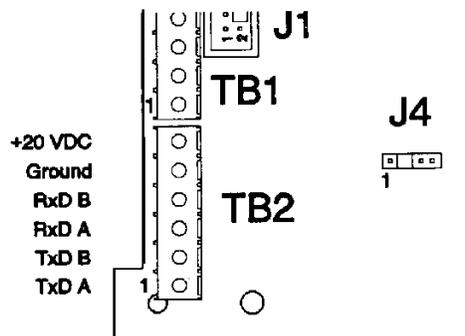
**Figure 6-8 - 8522 Main PCB Terminal Strip TB2**
