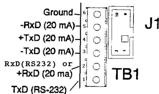
**Figure 6-14 - 8522 Main PCB Terminal Strip TB1**
