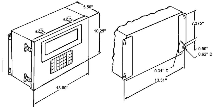
**Figure 3-1 - Wall Mount Enclosure Front and Rear Dimensions**
