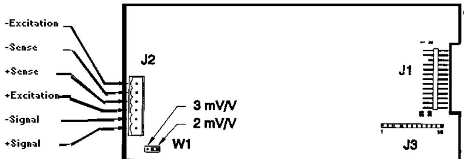
**Optional Analog Load Cell Input PCB (Desk Enclosure Versions)**
