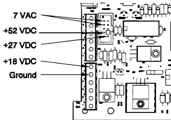
**Figure 7-1 - Main PCB Voltage Test Points**
