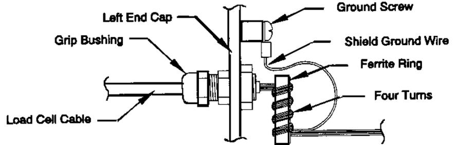
**Figure 6-11 - Ferrite Ring Installation**
