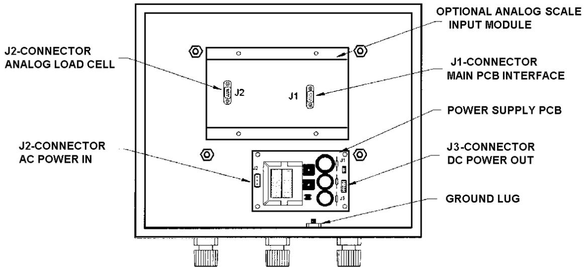
Figure 6-6 - Wall Enclosure Interior View
