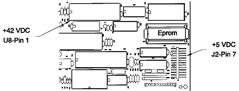
**Figure 7-2 - Main PCB, Voltage Test Points**
