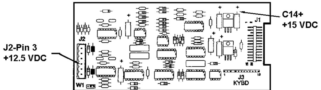
**Figure 7-3 - Analog PCB, Voltage Test Point Locations**
