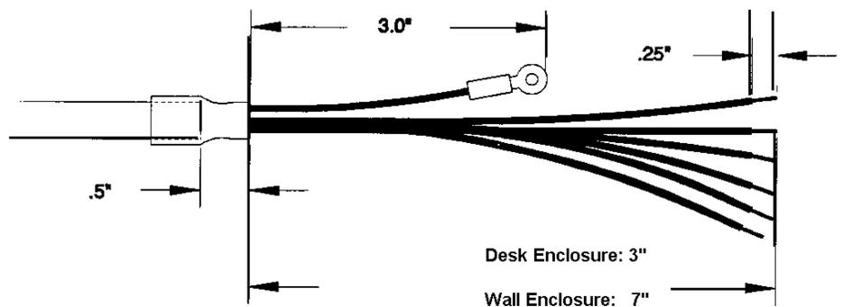
Figure 6-7 - DigiTOL<sup>®</sup> Load Cell Cable Preparation
