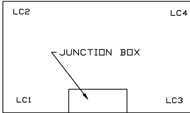
STANDARD FLOOR SCALE LOAD CELL ORIENTATION
