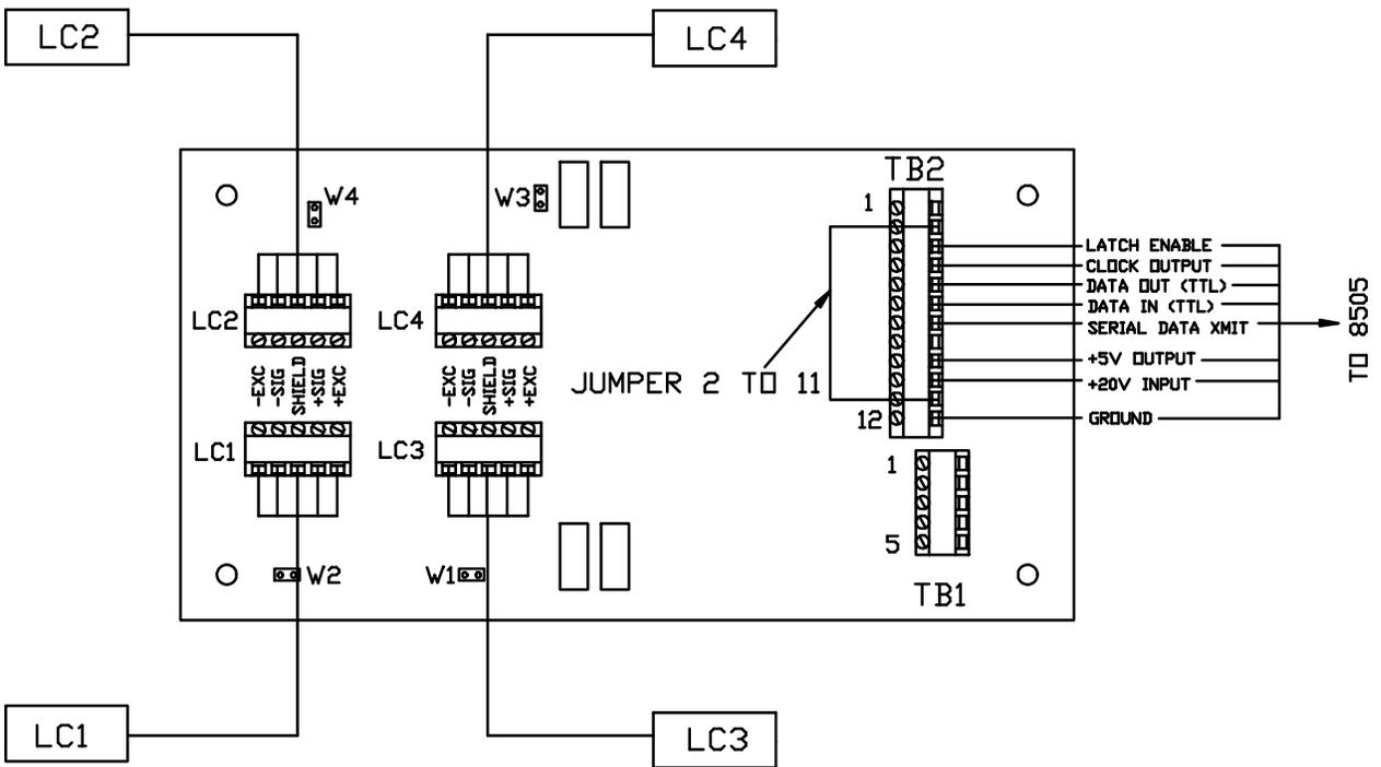
Figure 6-a Wiring Detail DLC Mode
