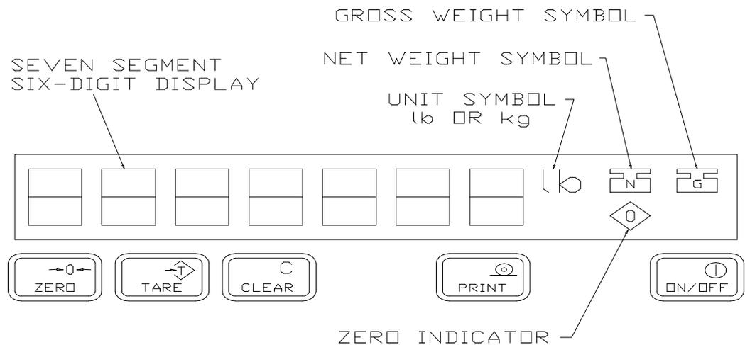
Figure 7-a Model 8505 Display Keyboard Layout
