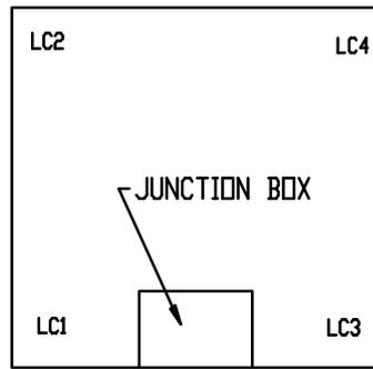
STANDARD FLOOR SCALE LOAD CELL ORIENTATION
