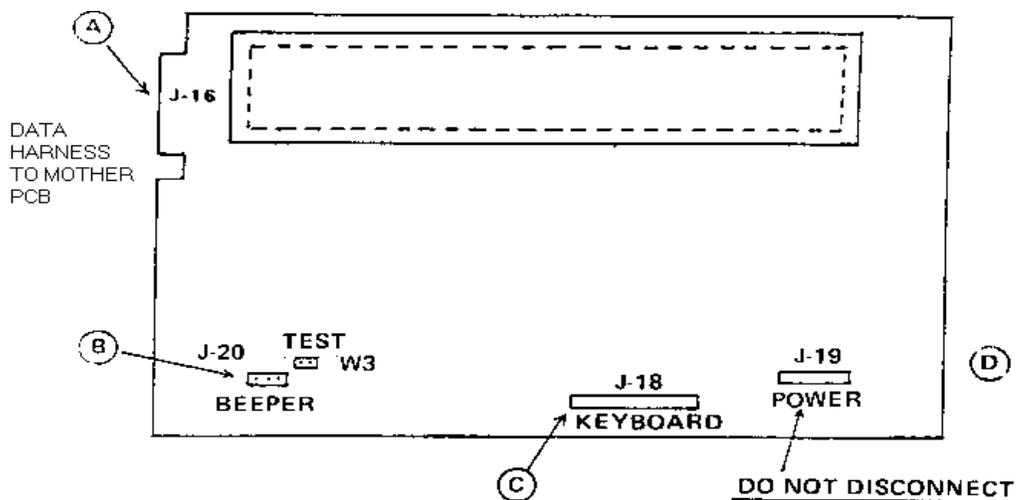
B and the keyboard harness C. Leave the power harness D connected.
