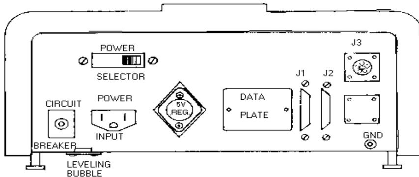
If the voltage selection switch requires changing, simply loosen the two retaining bracket until the selection switch is in the correct position for the voltage required and tighten the retaining bracket screws. See the figure above for clarification.
