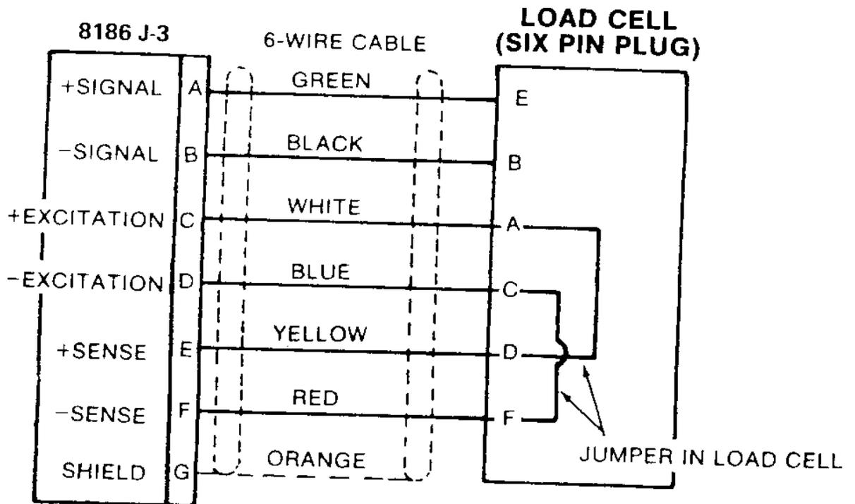
SINGLE 6 WIRE CELL CONNECTED DIRECTLY TO INSTRUMENT
