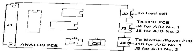
The Analog PCB contains no jumpers or program switches. Jacks are keyed at the following positions;
