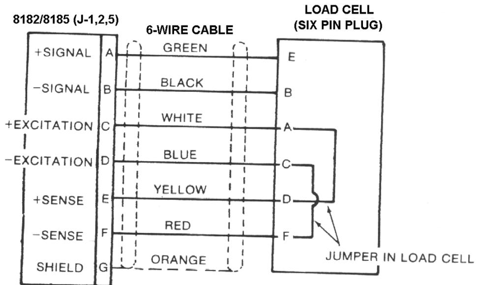
SINGLE 6 WIRE CELL CONNECTED DIRECTLY TO INSTRUMENT
