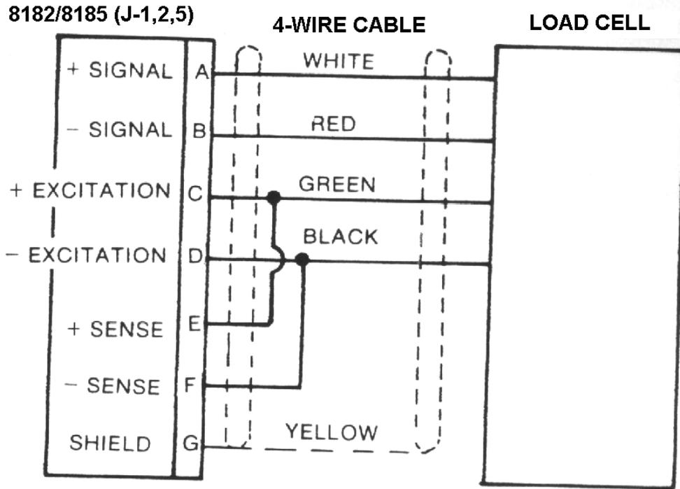
SINGLE 4 WIRE CELL CONNECTED DIRECTLY TO INSTRUMENT
