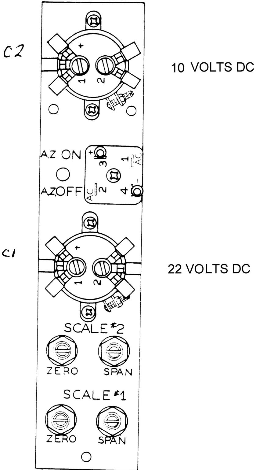
Observe polarity markings on capacitors.
