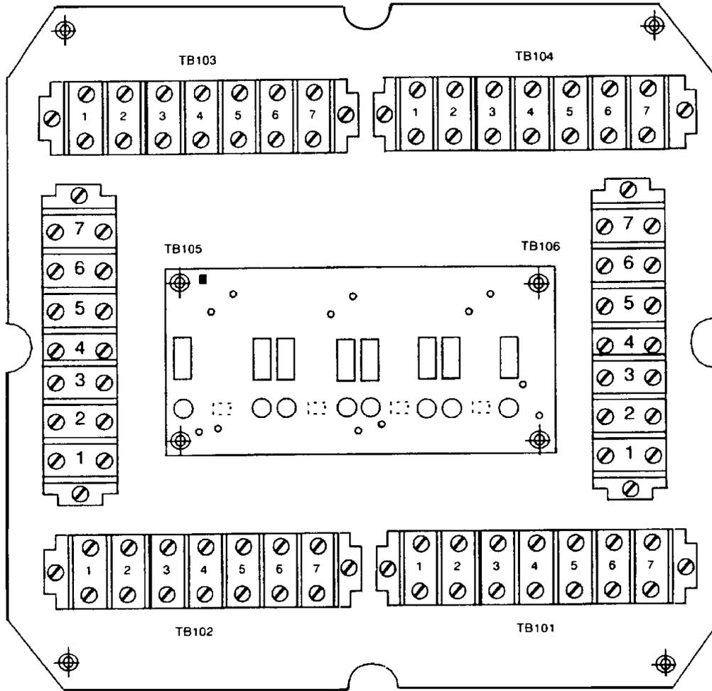
On terminal strips TB101\*, TB102, TB103, and TB104 a load cell is connected using the following guide. See Part 1 of this section for load cell color code.
