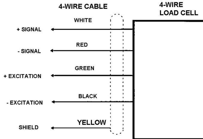
**NOTE:** When connecting a 4-wire load cell to the 8146, always jumper + excitation to + sense and - excitation to - sense at the junction closest to the load cell.
