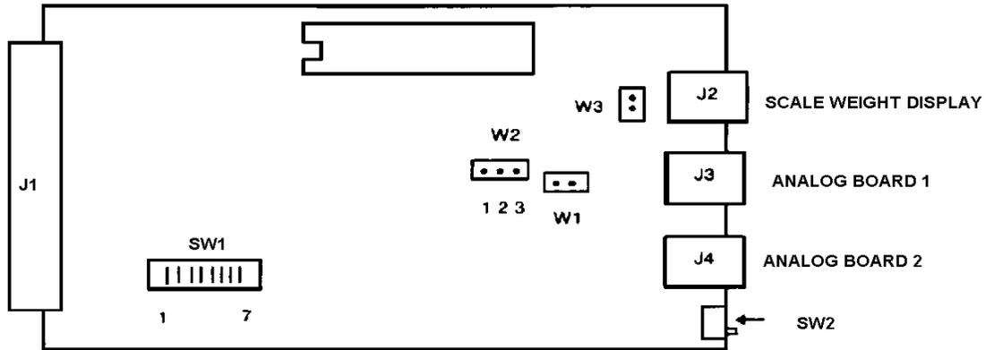
**SWITCH 1-1 ON - For the first Scale Channel PCB in the unit**
