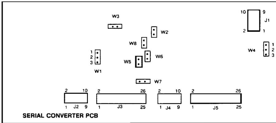
**W1 - Data Input Circuit Type (Keyboard/Display)**
