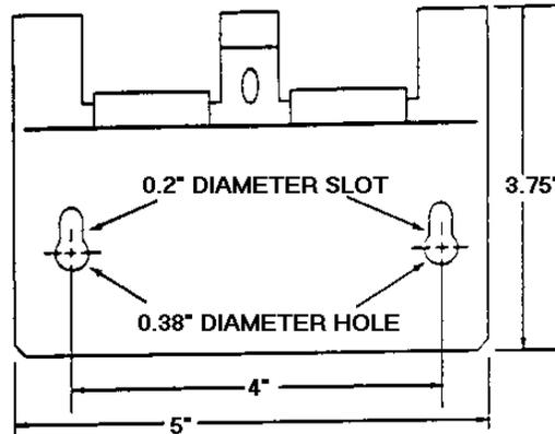
b. Mounting hole dimensions for wall mounting the stainless steel enclosure
