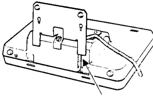
**ROUTE LOAD CELL CABLE THROUGH THIS CHANNEL**
