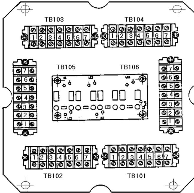
On terminal strips TB101\*, TB102, TB103 and TB104 a load cell is connected using the following guide. see part 1 of this section for load cell color code.
