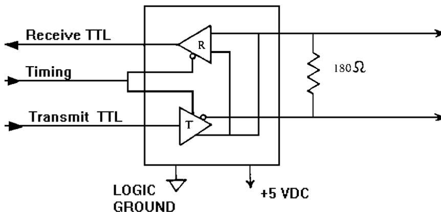
Interface to a "four-wire" scheme should not be required since the 8140 is not capable of receiving any data, only transmitting data. All data sent will be ASCII coded and transmitted at the baud rate selected in the data output setup. Step F12.
