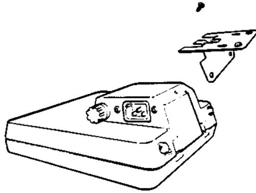
**NOTE:** Some Legal for Trade applications may require the removal of the Data Plate from the rear of the plastic enclosure and re-installation on the front. It should be installed on the lower left facing with non-conductive (plastic) fasteners.
