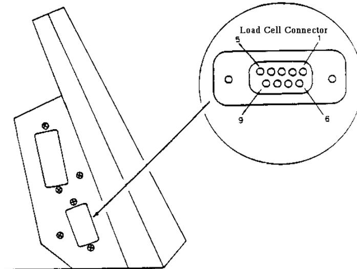
ii.) Secure the load cell cable or adapter harness to the J8 connector on the side of the enclosure. The pin configuration is shown.
