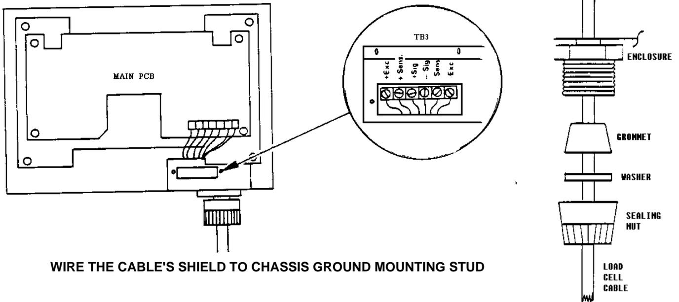
WIRE THE CABLE'S SHIELD TO CHASSIS GROUND MOUNTING STUD
