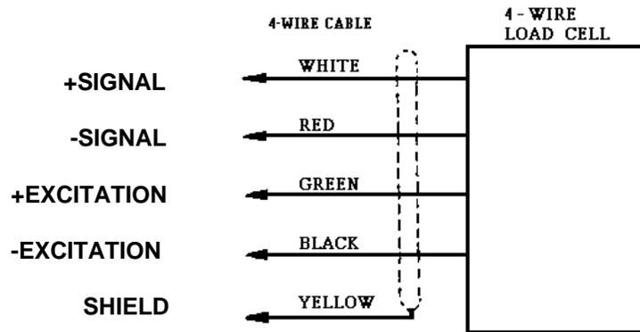
**NOTE:** When connecting a four wire load cell to the 8140, always jumper + excitation to + sense and - excitation to - sense at the junction closest to the load cell.
