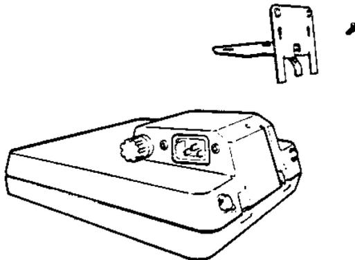
b. Bracket being installed for wall mounting.
