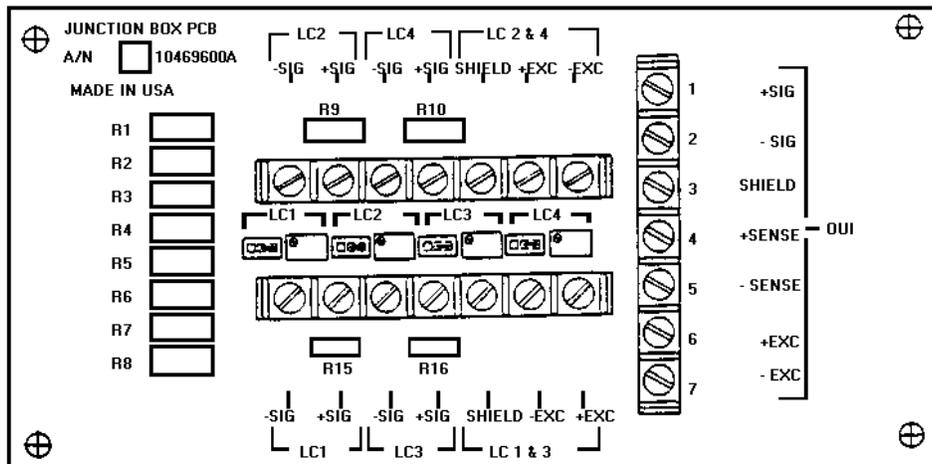
Terminal strip TB1 is the output terminal strip to the 8140 digital indicator. It should be wired as shown.
