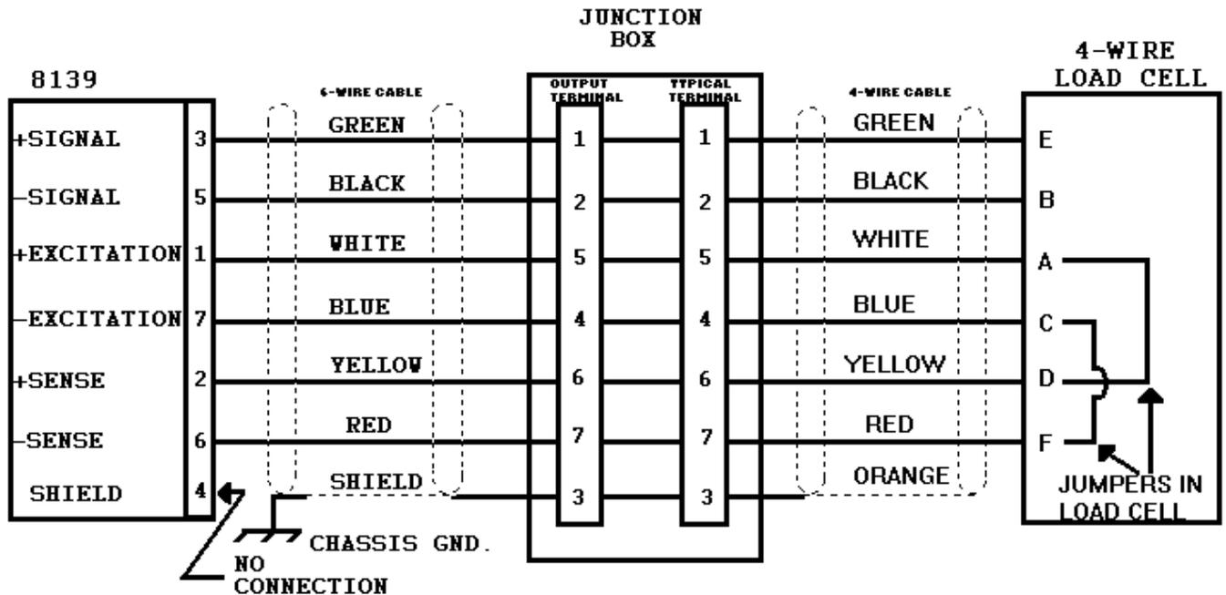
e). Typical single and multiple cell connections with a junction box.
