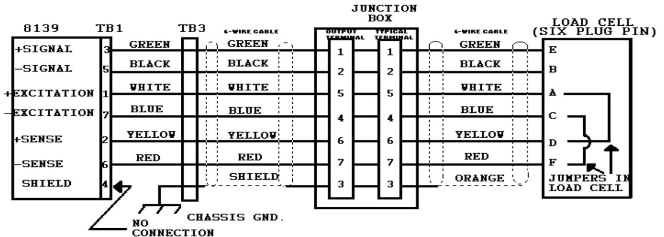
\* TB3 is the terminal strip on the bracket that contains the RFI filters on Rams 12, 13, 14, and 15. Ram 11 uses TB1 for these connections.
