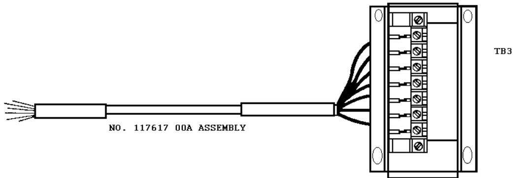
b). Typical single load cell connections:
