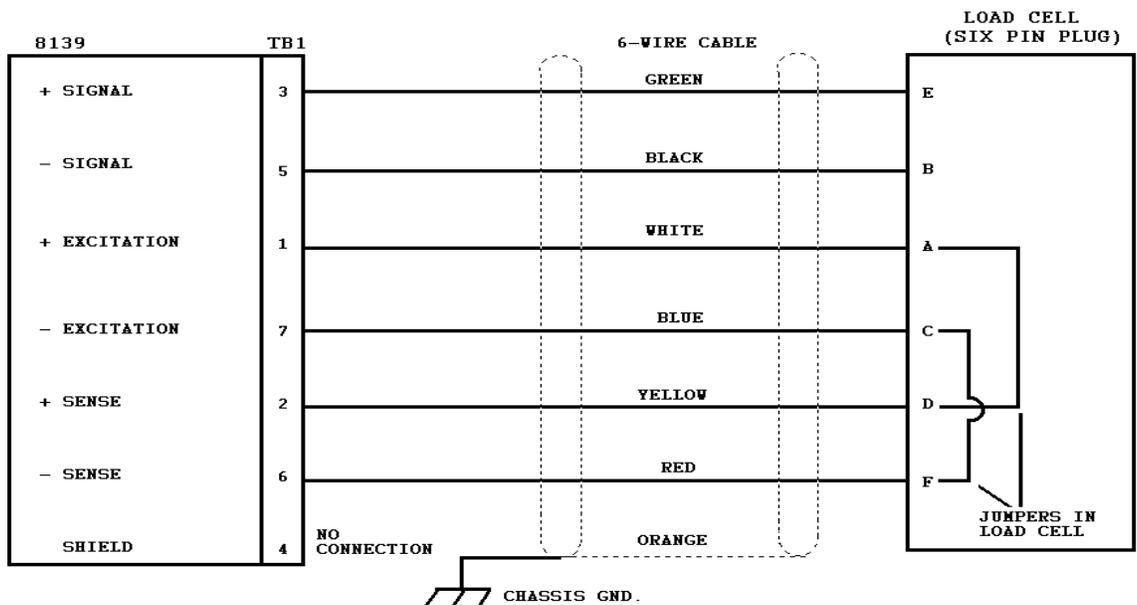
c). Typical single load cell connections:
