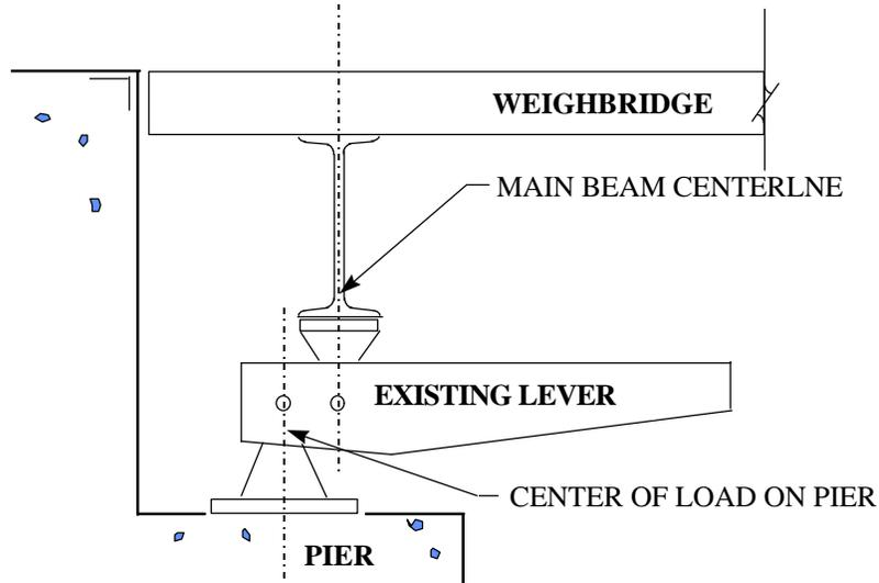
Figure 2-a: Typical Lever Corner Assembly
