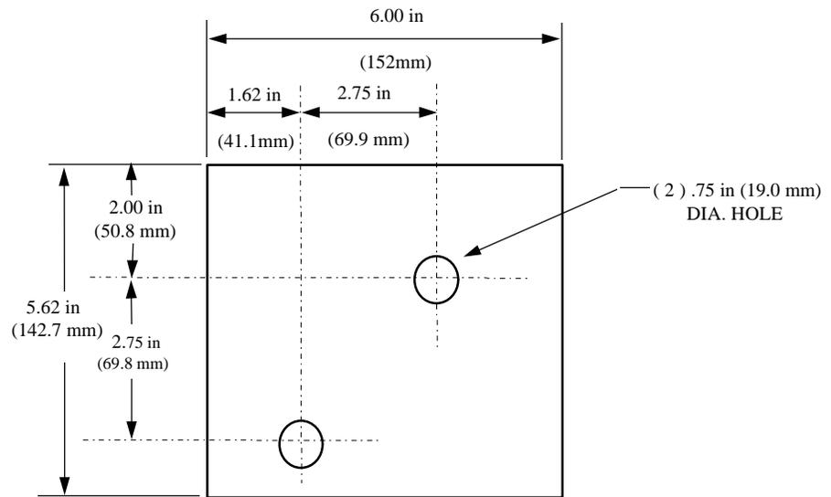
Figure 3-b: Leveling Shim Detail
