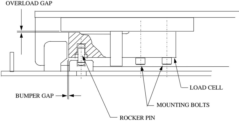
Figure 1-a: Load Cell Suspension Detail
