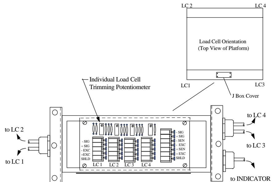
Figure 3-c: 2888 Analog Junction Box Details and Wiring Codes
