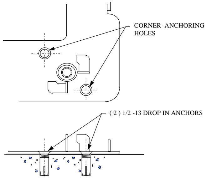
Figure 3-a: Frame Anchoring - Typical Each Corner
