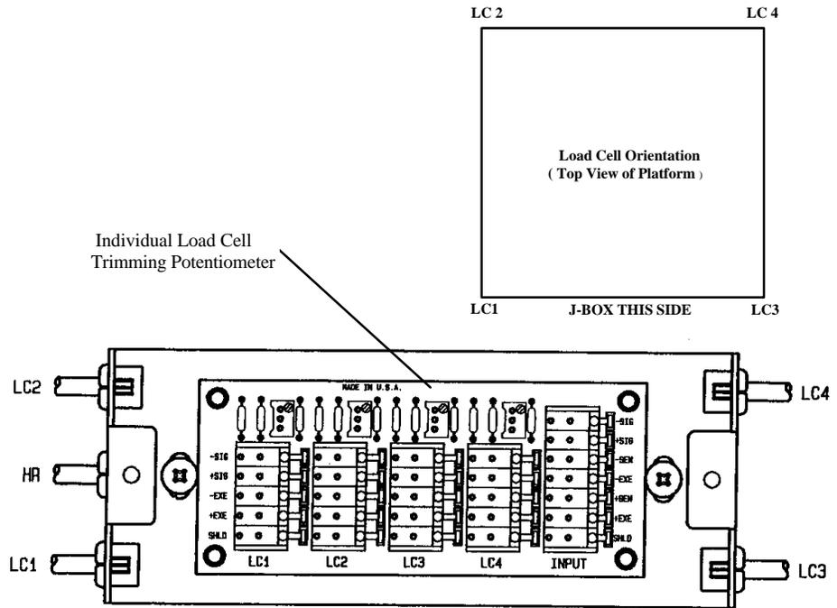
Note: Turn all potentiometers fully clockwise prior to calibration.
