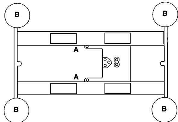
**Figure 4.2 Platter Support and Overload Stop Location**
