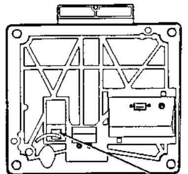
CAVITY FOR EXCESS CABLE
