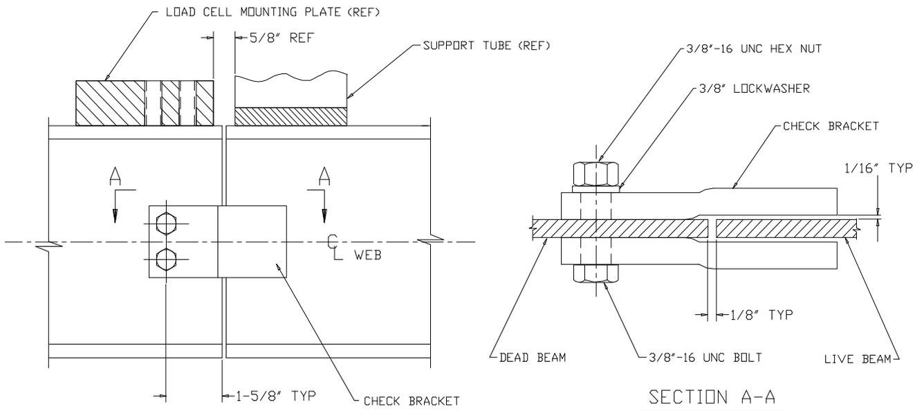
5.2.10 When you are confident the weigh modules are correctly positioned, run a continuous 1/4" fillet weld between the support tube and live beam and the load cell mounting plate and dead beam. Make sure the load cells have been removed before welding! **Use a certified welder to ensure a strong and safe weld.**
