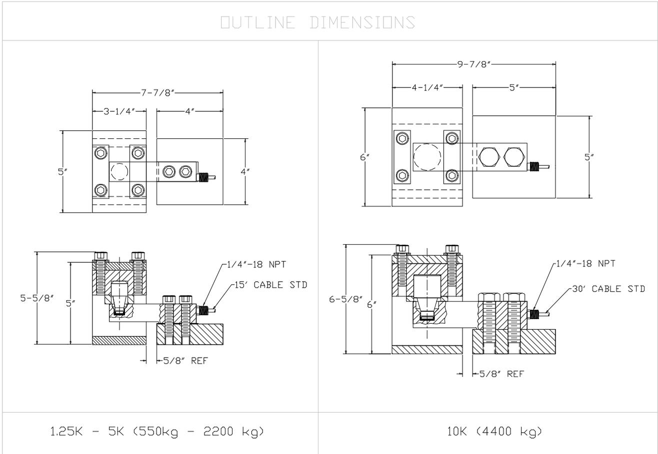
NOTE: "FIXED" MODULES ARE SHOWN. THE "SEMI-FLOATING" MODULES HAVE THE SAME DIMENSIONS.
