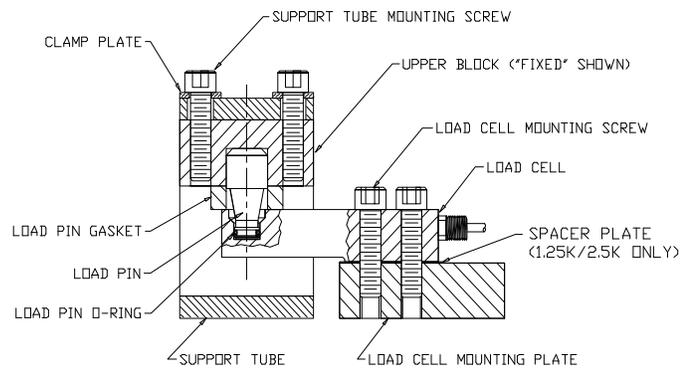
5.2.2 Place the assembled weigh modules on top of the existing I-Beam in the desired locations (See Figure 5.2).
