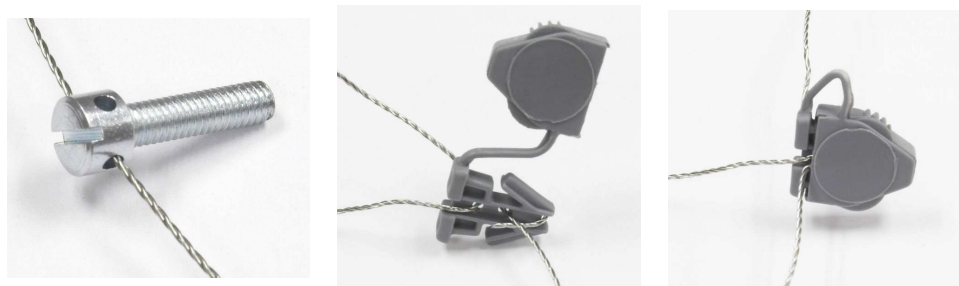
Figure 2-72: Use of the Sealing Kit: Wire Through Screw (left), Wire Through Seal (center), Seal Closed (right)
