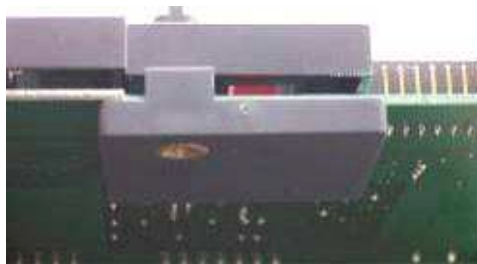
Figure A-56: Attaching the Plastic Bottom Sealing Plate
