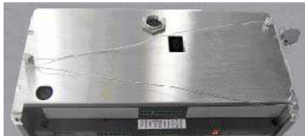
Figure A-54: External Sealing for Canada
