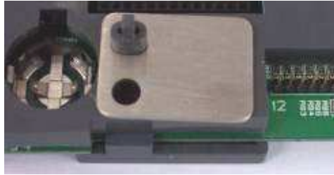
Figure A-57: Metal Sealing Plate
