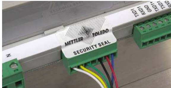
Figure A-60: Analog Load Cell Paper Seal
