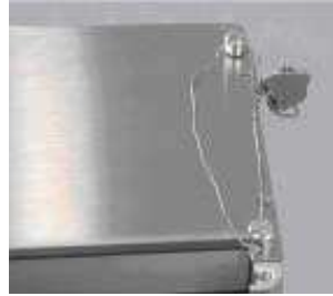
Figure A-53: External Sealing for United States
