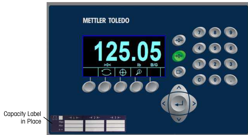
Figure A-51: Capacity Label Installed
