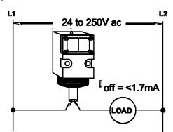
These sensors operate in the range of 24 to 250V ac, and may be programmed for either normally open (N.O.) or normally closed (N.C.) operation by way of the light-dark operate switch on the back of the sensor. A 2-wire ac sensor may be connected exactly like a mechanical limit switch.
