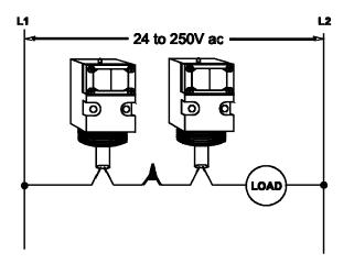
Most non-compatibility of series-connected sensors with loads occurs in low-voltage applications (e.g. 12, 24, or 48V ac circuits) where the on-state voltage drop across the load is a significant percentage of the supply voltage. The power-up inhibit time (up to 300 milliseconds per sensor) is also additive.
