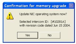
TalkMaster will connect to the Intercom and begin uploading the firmware. When the upload is completed, a dialog box will be presented informing you that the action was successful. Once you click OK, the screen will lock for 30 seconds while the firmware re-programming takes place.
